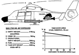
Fig. 24 MAD - TORPEDOES INSTALLATION
