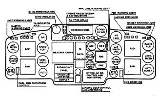
Fig. 11 SA 365 F INSTRUMENT PANEL MULTIFUNCTION DISPLAY CONFIGURATION
