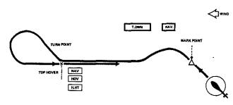
Fig. 7 APPROACH OF A MARKED POINT
