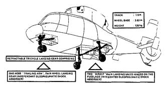
Fig. 3 SA 365 F LANDING GEAR
