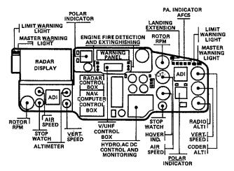
Fig. 10 SA 365 F INSTRUMENT PANEL ELECTRO-MECHANICAL FLIGHT INSTRUMENTS
