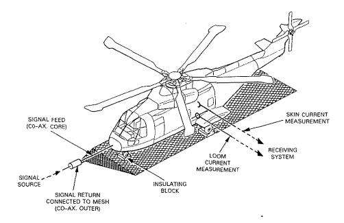
With a swept-frequency c.w. signal applied to the aircraft, the skin currents and loom currents are measured with the surface- and loom-current probes.
