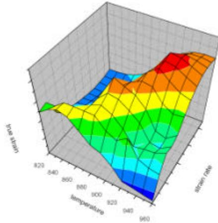
Figure 4: 3-D-plot of “Cone Cup Test”-results for SPF-parameter selection
