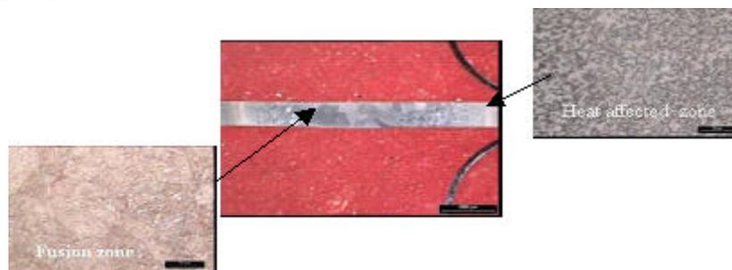
Figure 10: LBW of SPF`ed Ti6-2-4-2 to Ti6-2-4-2 in as-received condition
