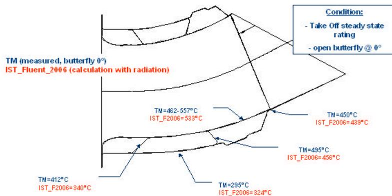
Figure 16: Second campaign result. Validation of temperature simulation with measured data
