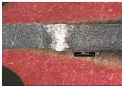
Figure 12: LBW of SPF'ed beta21S welded to beta21S in as-received condition without  $H_2$  contamination
