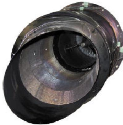
Figure 14: Exhaust nozzle after first campaign with Max Take off Power (MTP)
