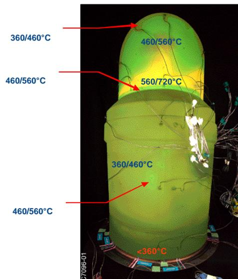
Figure 15: First campaign. Exhaust nozzle after coloration test at MTP
