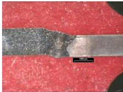
Figure 13: LBW of SPF'ed Ti6-2-4-2 welded to Hot formed beta21S
