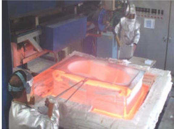
Figure 6: SPF-die for the exhaust skin half shell in action
