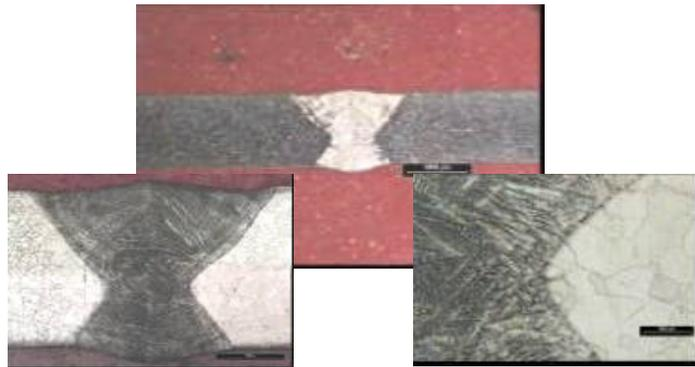
Figure 11: LBW of SPF'ed beta21S to beta21S with  $H_2$  contamination
