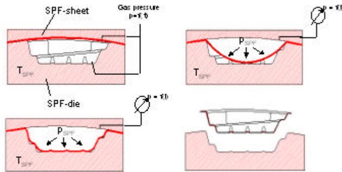
Figure 2: Forming with gas pressure under elevated temperature
