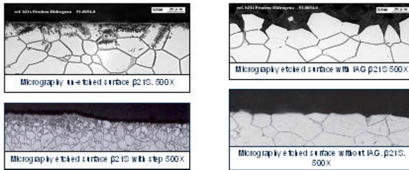
Figure 8: Different surface smoothness as a function of the chemical-mill process
