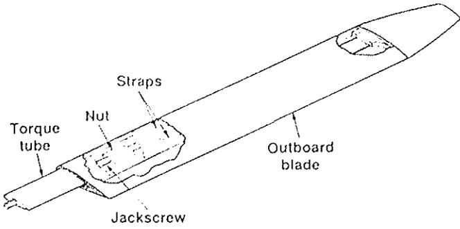
Figure 32 - Telescoping Rotor Blade Schematic
