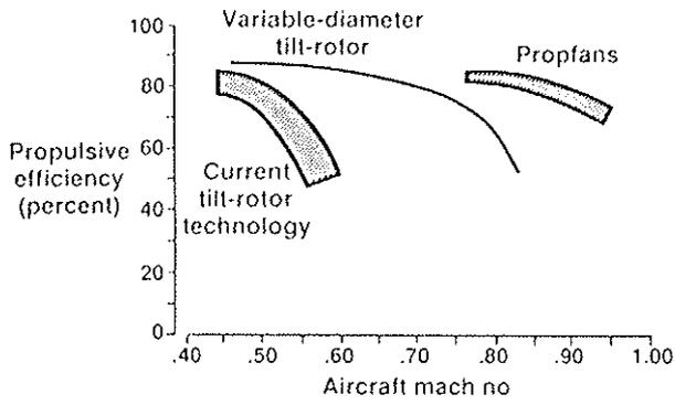
Figure 38 - Maximum Propulsive Efficiency vs. Flight Mach No.
