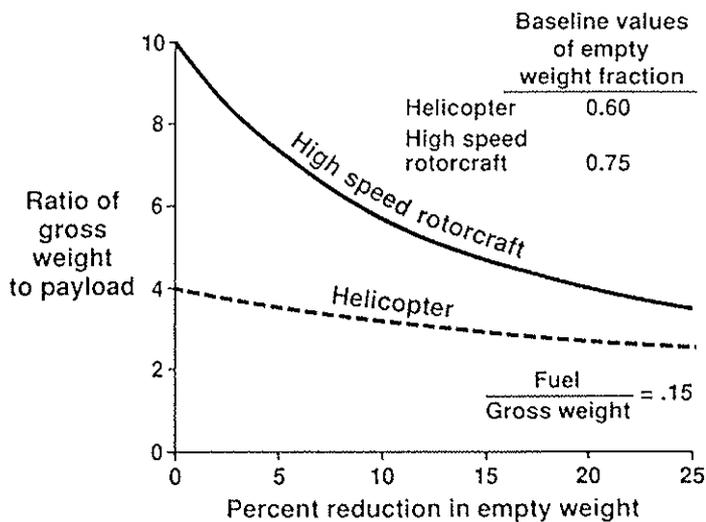
Figure 40 - Effect of Empty Weight Reduction on Gross Weight
