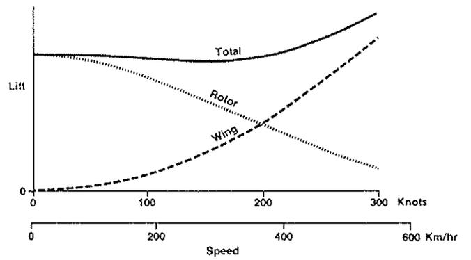
Figure 5 - Combined Lift of Rotor and Wing
