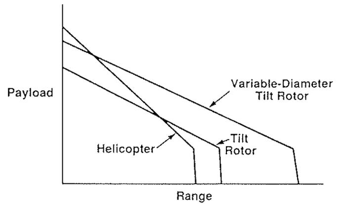
Figure 42 - Variable Diameter Improves Tilt-Rotor Payload/Range Characteristics
