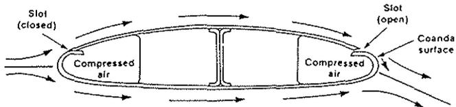
Figure 27 - X-Wing Airfoil with Circulation Control
