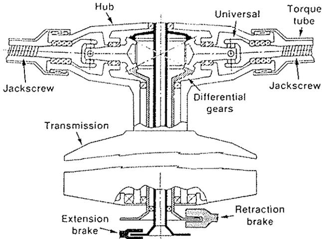
Figure 33 - Retraction Mechanism Schematic Arrangement
