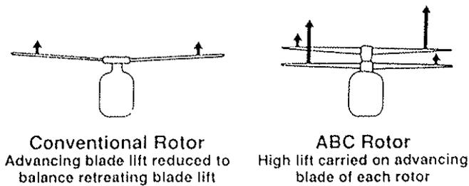
Figure 10 - Basic Principle of Advancing Blade Concept
