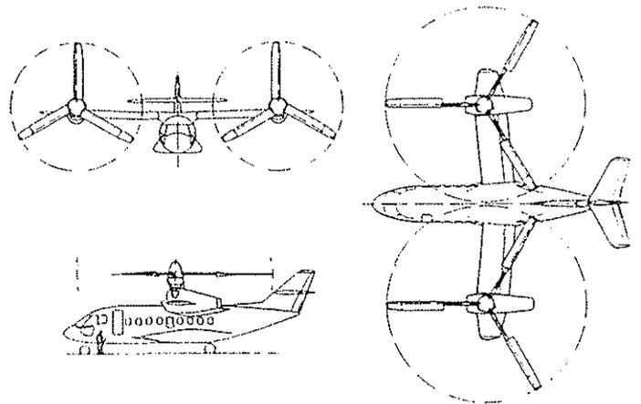
Figure 37 - Variable-Diameter Tilt-Rotor Aircraft
