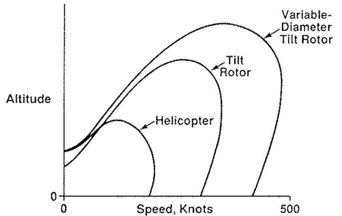
Figure 43 - Variable Diameter Expands Potential Tilt-Rotor Flight Envelope
