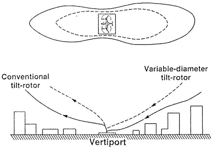
Figure 45 - Variable Diameter Will Reduce Acoustic Footprint
