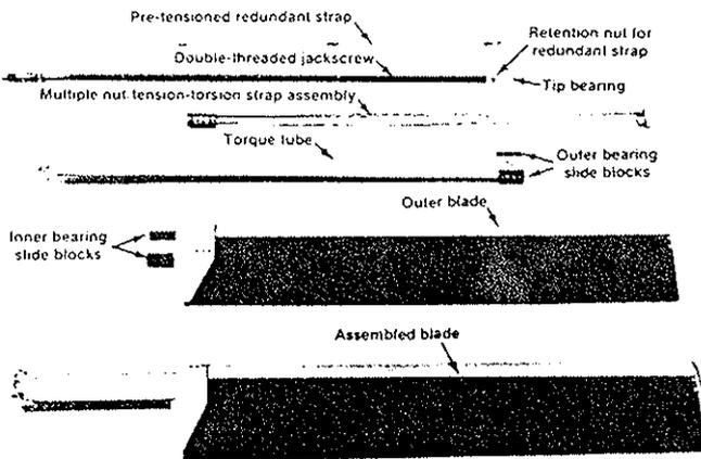
Figure 34 - Wind Tunnel Model Blade Components
