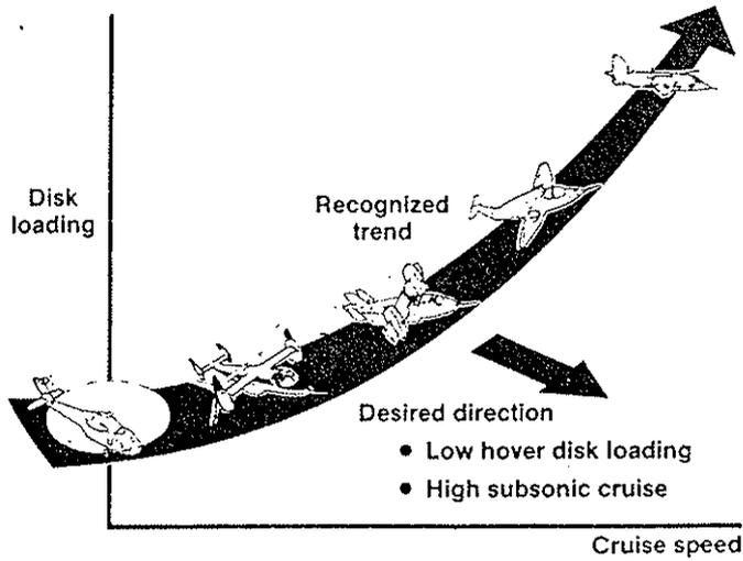
Figure 2 - Disk Loading-Cruise Speed Trends
