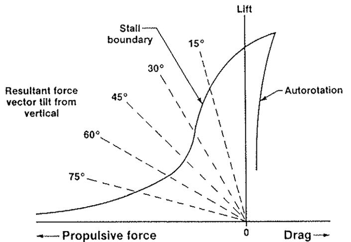
Figure 13 - Typical Rotor Aerodynamic Envelope Limits Over Full Tilt Range
