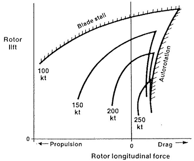
Figure 4 - Effect of Speed on Rotor Force Capabilities
