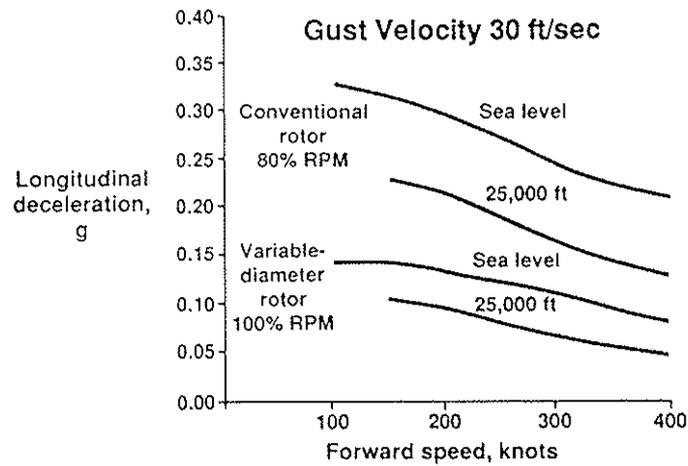
Figure 46 - Variable Diameter Reduces Response To Head-On Gust
