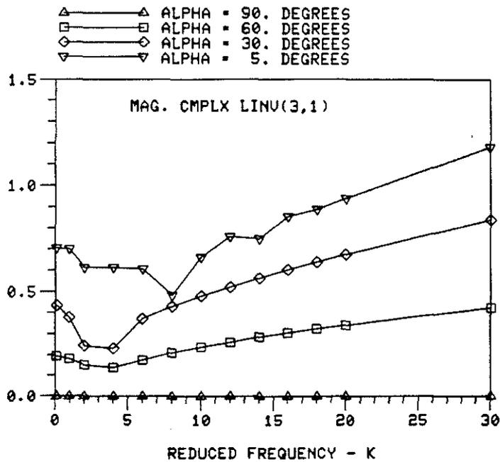
Figure 5. Magnitude of the (3,1) Element of Inverted Complex L(K) Matrix for  $\alpha$  Sweep (Corrected Pressure)
