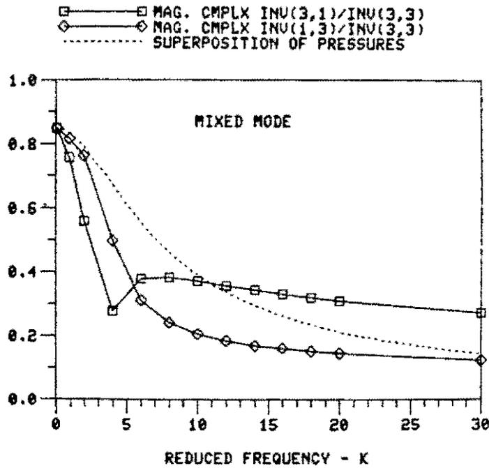
Figure 7. Relative Magnitude of the Off-Diagonal Terms of the 3X3 Inverted Complex L(K) Matrix at  $\alpha = 30^\circ$
