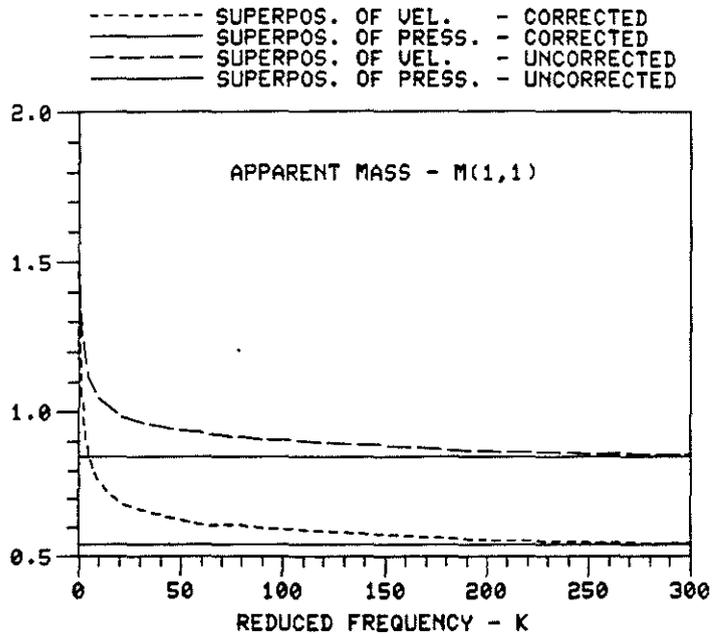
Figure 2. Apparent Mass Element M(1,1) for  $\alpha = 90^\circ$
