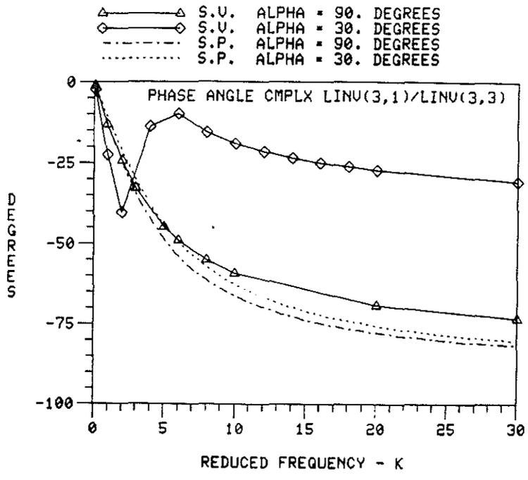
Figure 8. Phase Angle of Complex (3,1)/(3,3) for Analytical L and M Matrices
