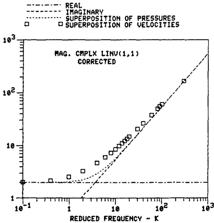
Figure 3. Magnitude of the (1,1) Element of Inverted Complex L(K) Matrix at  $\alpha = 90^\circ$  with Corrected Pressure
