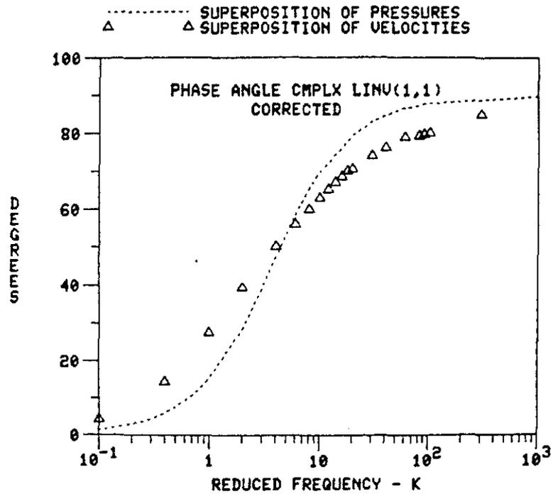
Figure 4. Phase Angle of the (1,1) Element of Inverted Complex L(K) Matrix at  $\alpha = 90^\circ$  with Corrected Pressure Distribution
