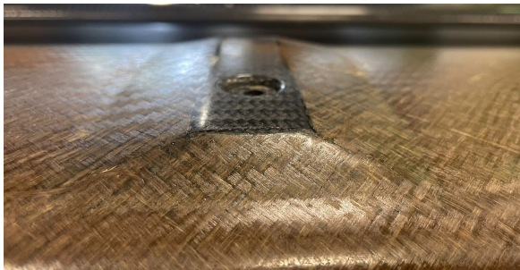
Fig. 40: Attachment area on the underside of the hybrid horizontal stabilizer
