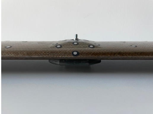
Fig. 33: Bulge for reinforcement around the clamping of the horizontal stabilizer
