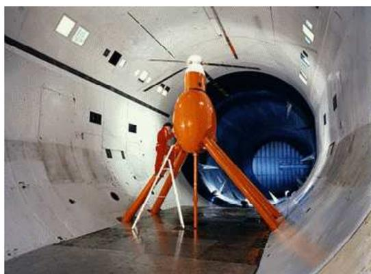
**Fig. 1. 7A rotor mounted in the ONERA Modane S1MA Wind Tunnel.**
