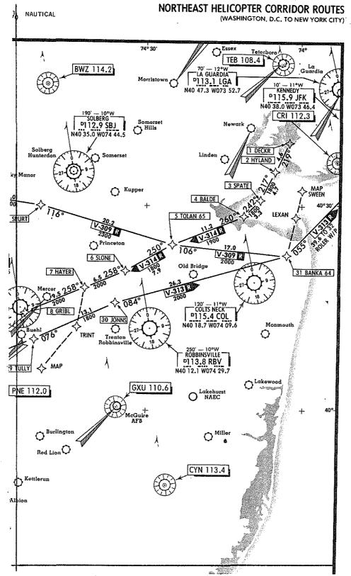
Portion of U.S. Northeast Corridor connecting Washington and Boston by discrete helicopter RNAV routes. GPS RNAV would provide highly accurate, narrow route widths on this type of RNAV route structure.
