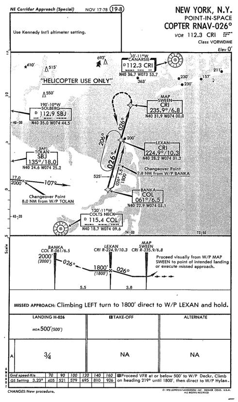
Helicopter Point-In-Space RNAV instrument approach procedure for flight from the south/southwest into the New York area. GPS RNAV would permit highly accurate flight paths, a low MDA, and minimum airspace requirements for both approach and missed approach procedures.
