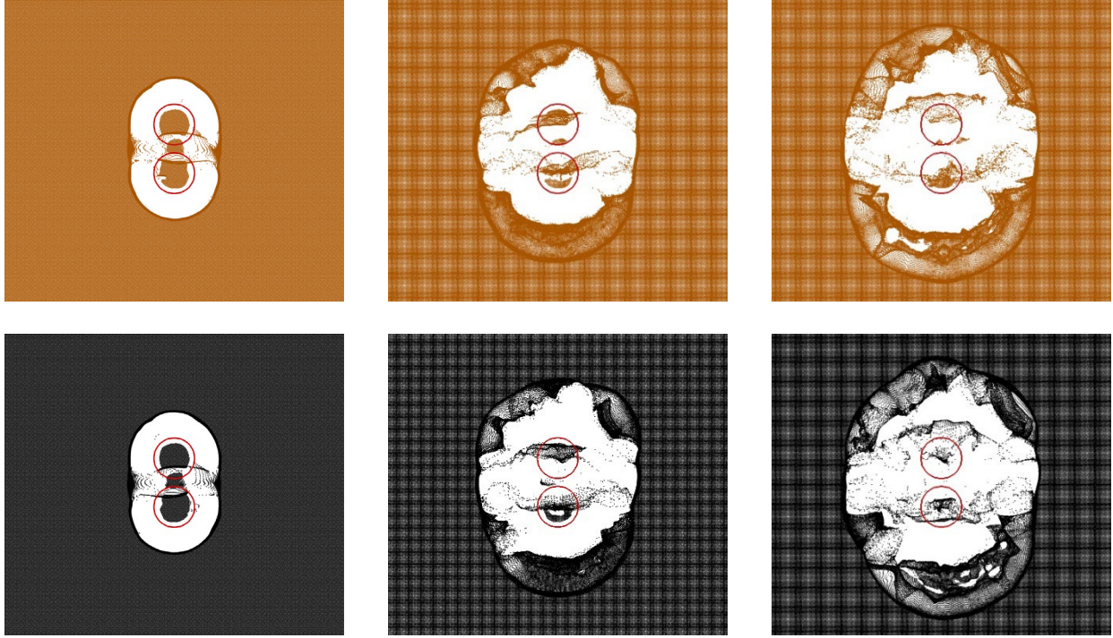
Figure 32: Top view of the time evolution, from left to right, of the brownout cloud generated by side-by-side counter-rotating rotors (top) and co-rotating rotors (bottom) after 1.5s; 2.5s; and 3s, respectively.
