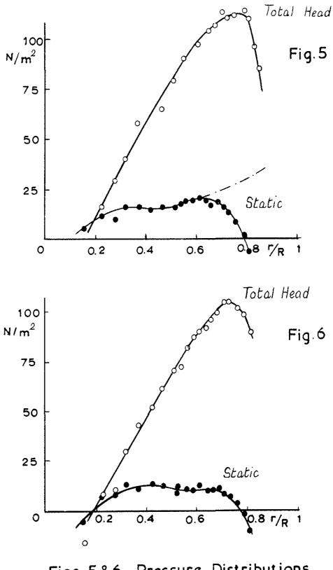
Figs. 5&6 Pressure Distributions (Rotor B)
