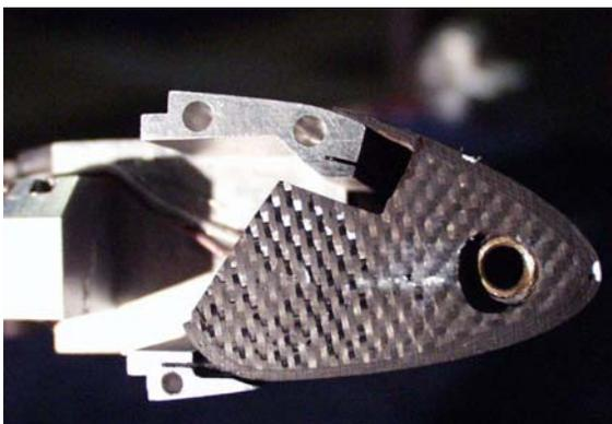
Fig.3: Movable Leading Edge, Side-View
