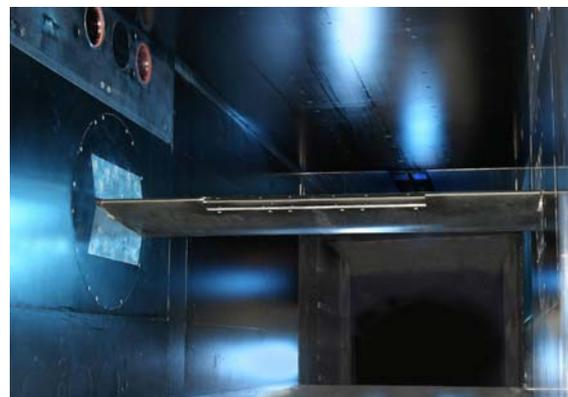
Fig.1: Model in DNW-TWG test section
