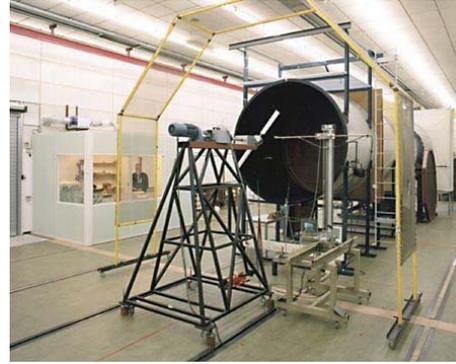
Figure 2 – The model wind turbine and open jet wind tunnel used
