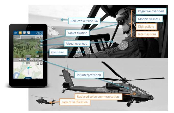
Figure 2: potential negative effects on the flight crew
