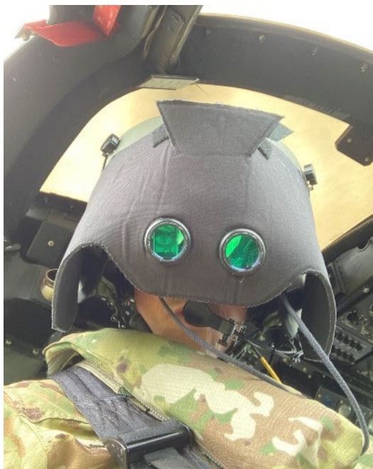
Fig. 8. Hood and filtered NVGs produce UCE 2
