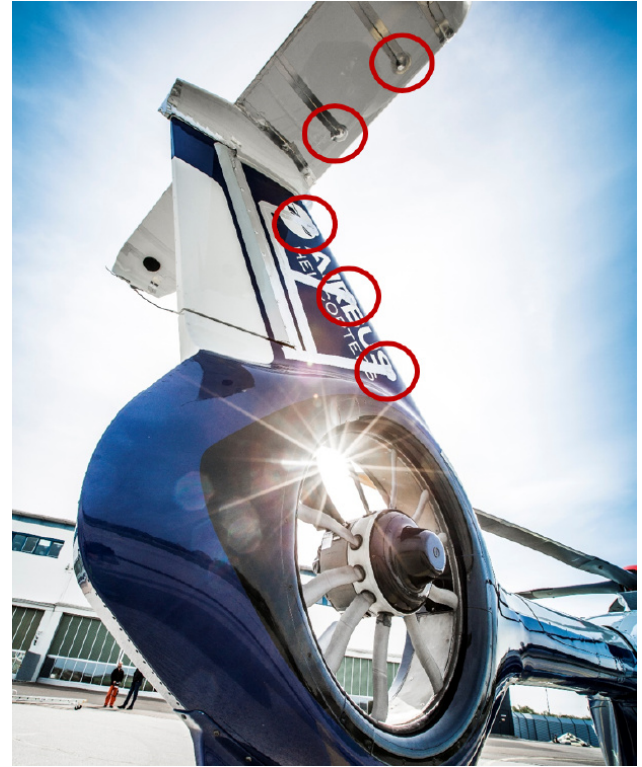
Fig. 4: Pressure sensor instrumentation at the Bluecopter™ empennage [21]
