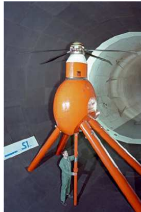
Fig. 2. ERATO rotor mounted in the ONERA Modane S1MA Wind Tunnel.
