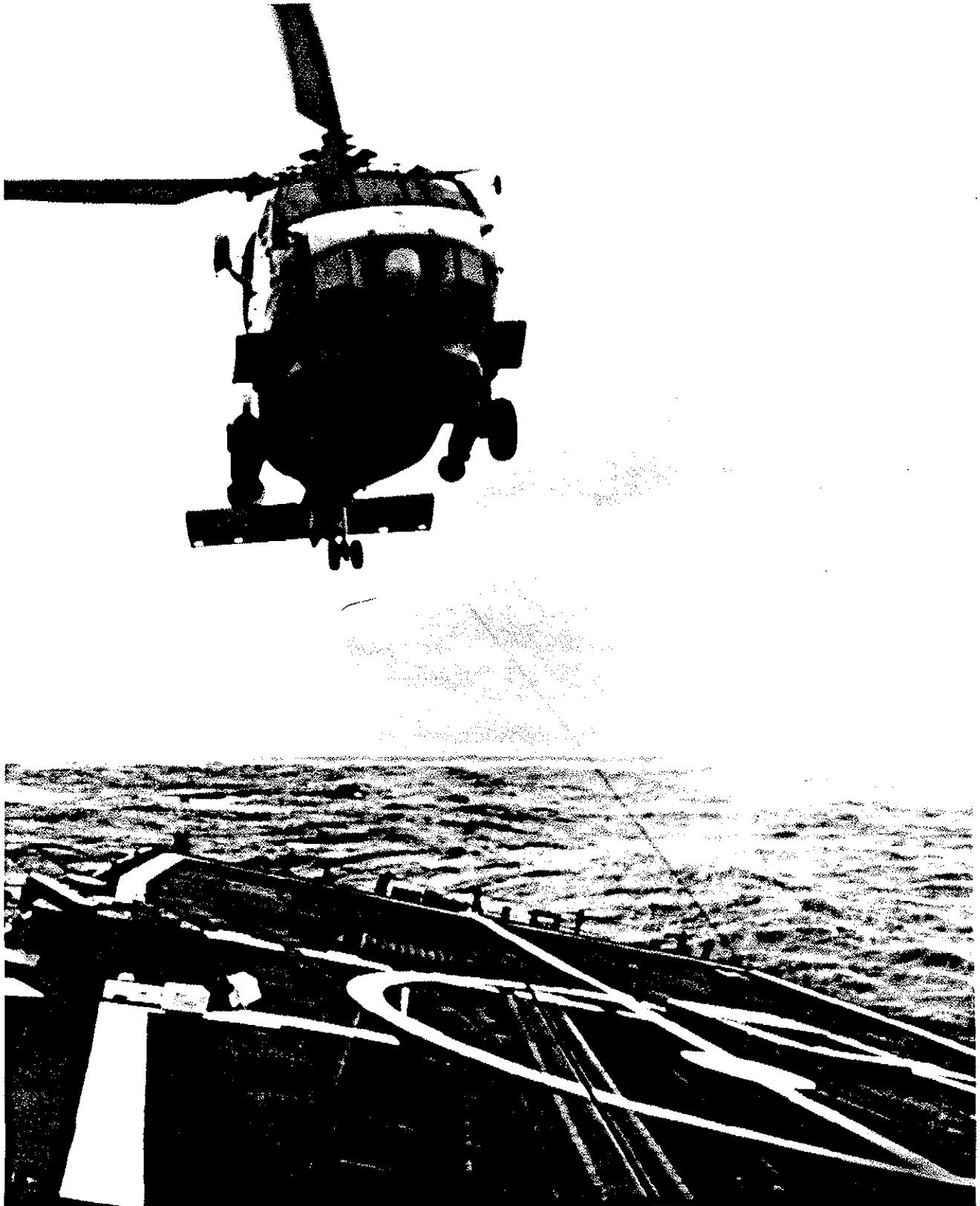
Illustration 12. The RAST (Recovery, Assist, Secure and Traverse) system at work in a USN FFG with the Sikorsky SH-60B Sea Hawk on the wire.
