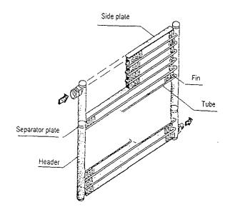
Fig 6-1 - Flat Tube and Fin Condenser Schematic
