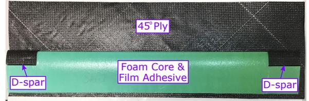
**Fig. 2: Main components used for fabrication of the composite blade**
