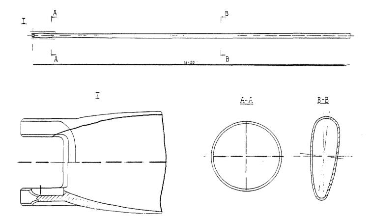
Fig. 3. Steel spar for Mi-26 main rotor blade.
