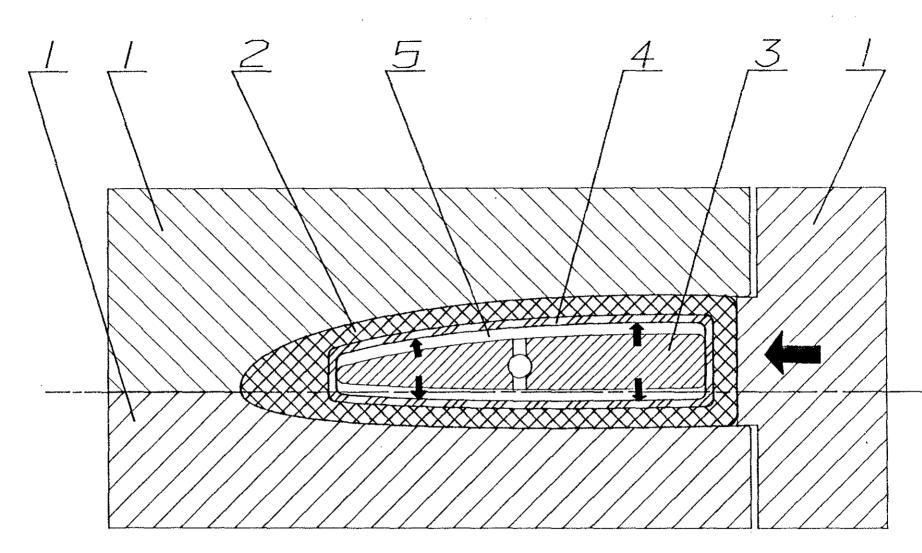
Fig.6. Schematic diagram of facility for curing composite blade spars.
