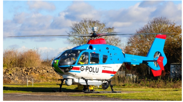
Figure 5: BladeSense ground runs: H135 helicopter with hub support cap and instrumented blades during a ground run.
