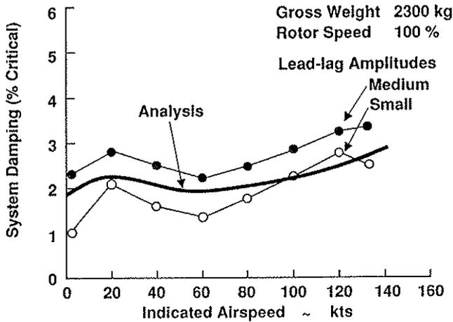
Fig. 17 Air resonance stability (rotating system)
