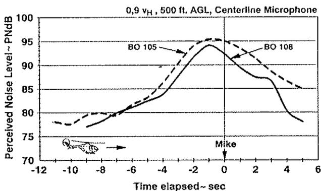
Fig. 18 External noise measurement
