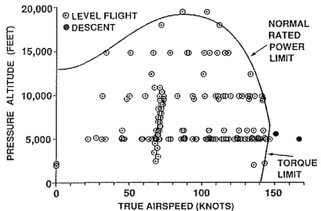
Fig. 14 Prototype 1 flight test envelope
