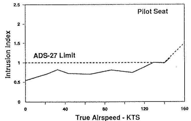
Fig. 16 Fuselage vibrations vs. airspeed
