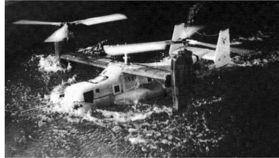
**Fig. 27. Scale model water impact test.**
