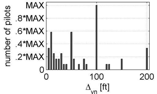
Figure 16: Distribution of the minimum accepted vertical clearance  $\Delta_{vn}$  during takeoff
