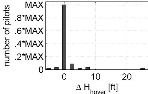
Figure 14: Differences  $\Delta H_{hover}$  between hover height  $H_{hover}$  used and flight manual advisory  $H_{hover}^{FM}$
