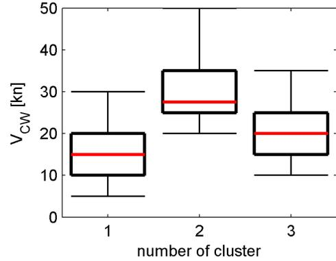
Figure 24: Maximum accepted crosswind  $V_{cw}$
