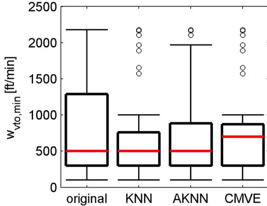
Figure 20: Exemplary result of imputation for the rate of climb used for NTO
