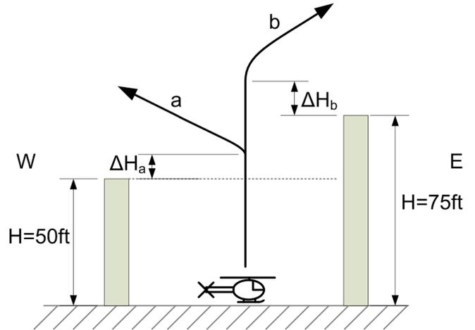
Figure 2: Example of a depiction showing different ways to leave a confined area
