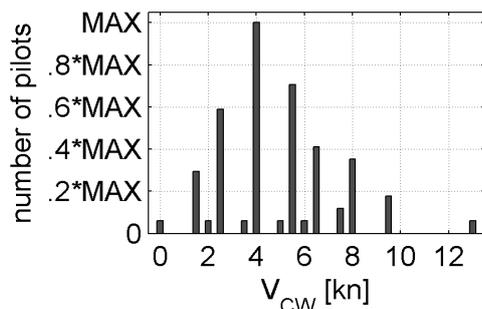
Figure 15: Distribution of the maximum accepted crosswind  $V_{cw}$  during takeoff
