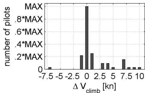
Figure 13: Differences  $\Delta V_{climb}$  between speed flown during climb  $V_{climb}$  and typical climb speed  $V_Y$  taken from the flight manual
