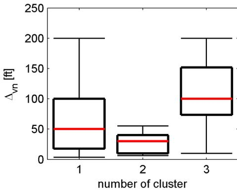
Figure 23: Vertical clearance to obstacles for normal takeoff  $\Delta_{vn}$
