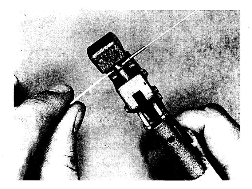
Figure 8. Crimping of Connector Alignment Ferrule
