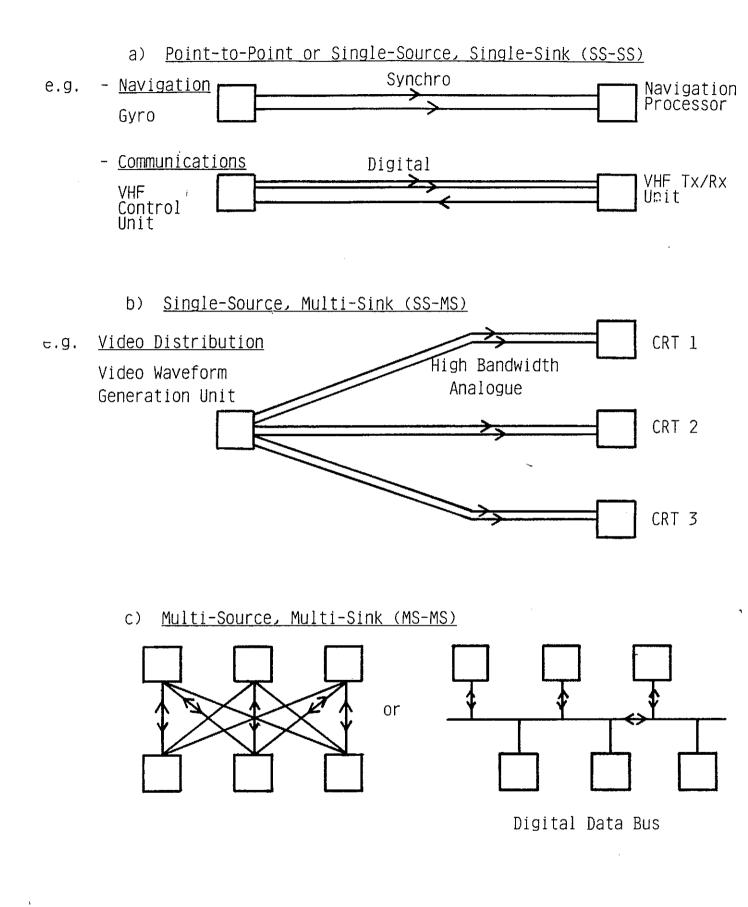
Figure 1. Aircraft Data Transmission Architectures
