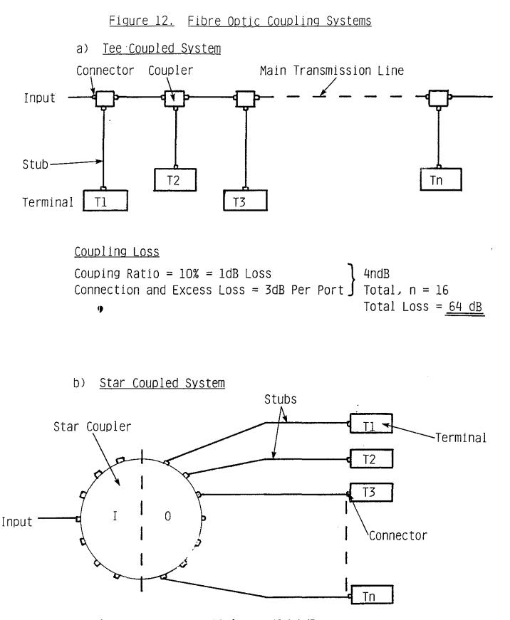
Coupling Ratio =  $\frac{1}{n}$  = 10 log<sub>10</sub> (1/n)dB Excess Loss for Any Port = 3dB 3 + 10 log<sub>10</sub> (1/n) dB n = 16 (15dB)
