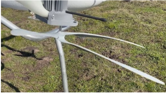
Figure 1 Asymmetric “Hummingbird” propeller by Zipline. The photo is taken from a video by Mark Rober 2 .
