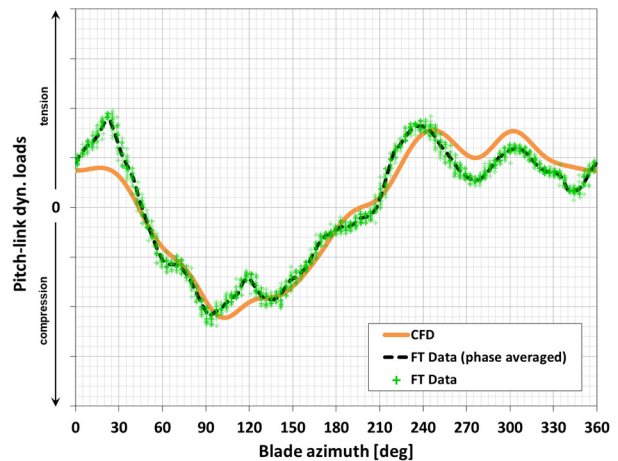
Figure 13 – Dynamic loads at pitch link as a function of the blade azimuth \psi for LEVEL_REF_SER
