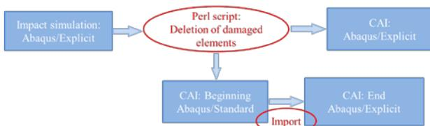
**Figure 23:** CAI execution via Abaqus/Explicit and Standard
