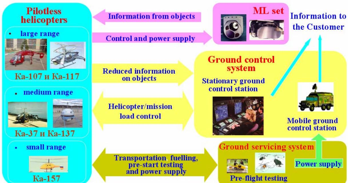
**Fig. 8 Configuration and functional relations of rotary-wing UAV systems**
