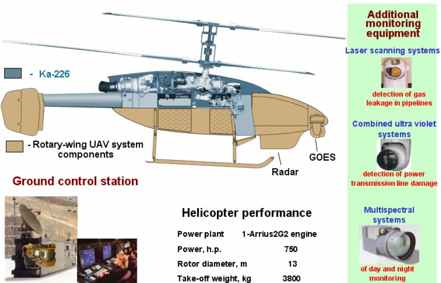
**Fig. 11 Long-range rotary-wing UAV layout**
