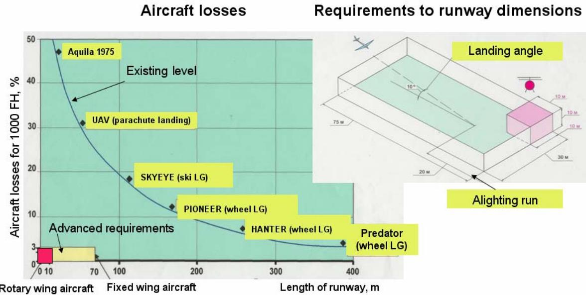
**Fig. 2. Unmanned aircraft take-off and landing**
