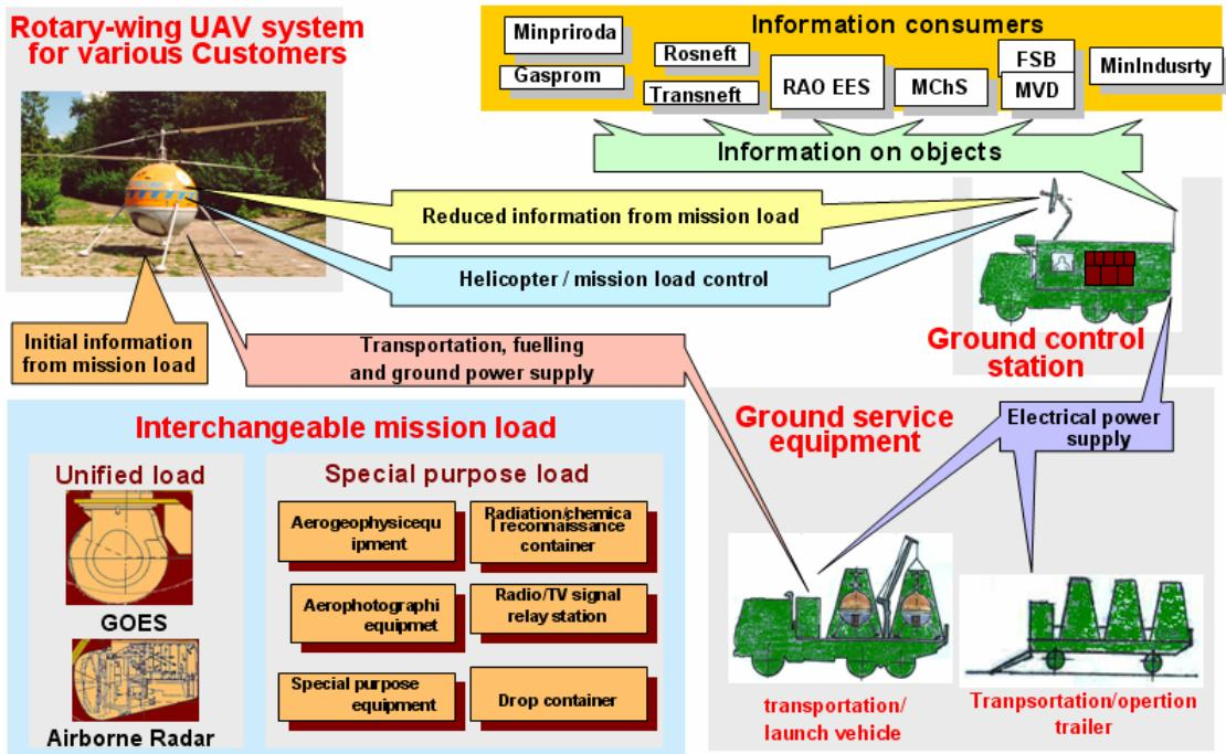
*Fig. 12 Configuration and functional relations of a medium-range rotary-wing UAV system*
