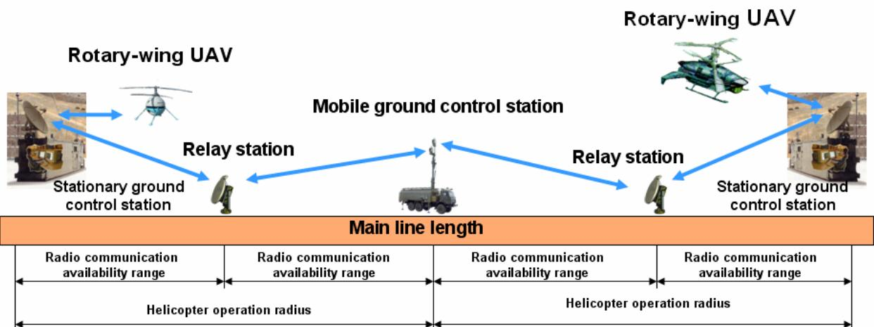
**Fig. 7 Pattern 3. Monitoring of main line (network) of large length using a mobile/permanent ground control stations and intermediate relay stations**
