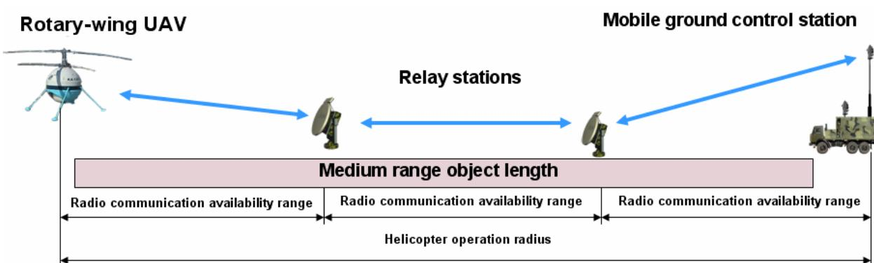
**Fig.6 Pattern 2. Monitoring of regional objects (network) of average length using a mobile ground control station and intermediate relay stations**
