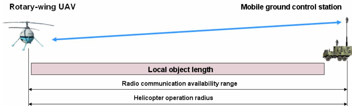
**Fig. 5 Pattern 1. Local object (network) monitoring by an integrated system with a mobile ground control station**
