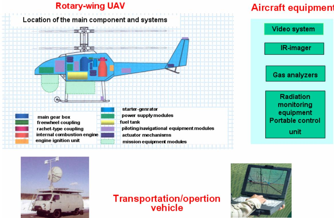
*Fig. 14 Short- range rotary-wing UAV system*
