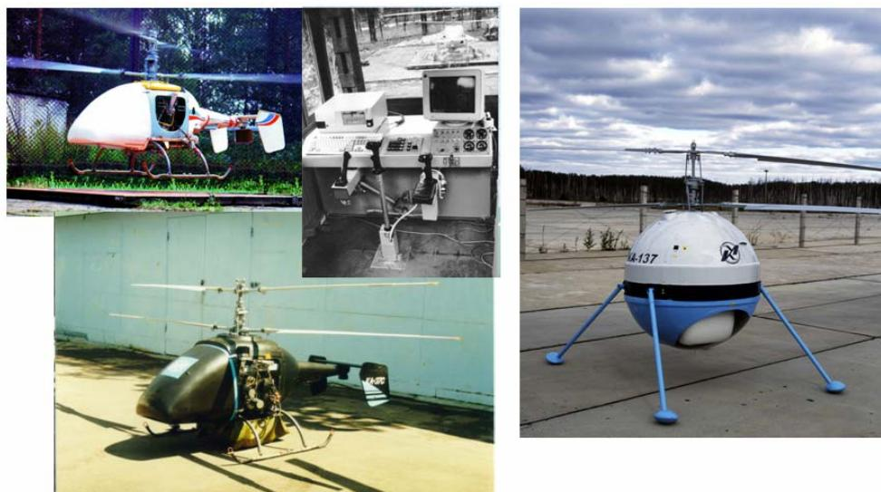
*Fig. 13 Verification of a medium-range rotary-wing UAV elements on the Ka-37 flying test bed and the Ka-137 mock up*
