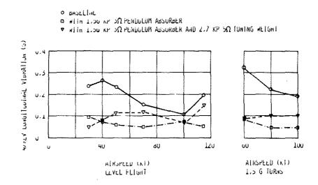
Figure 14: Effect of 3/rev pendulum absorber and 5/rev tuning weight on 4/rev lateral vibration
