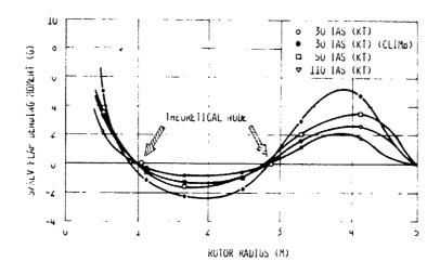
Figure 4: Correlation between 5/rev forced vibration and mode shape due to 3<sup>rd</sup> flap bending natural frequency
