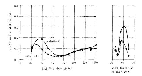
Figure 21: Effect of mass tuning on 4/rev vertical cabin vibration
