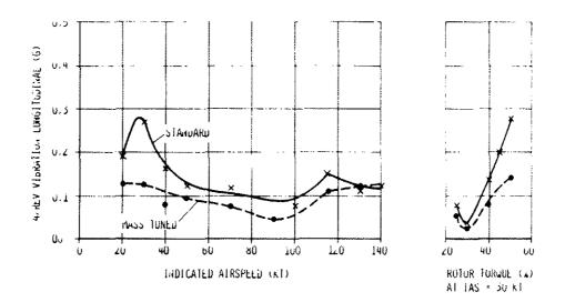
Figure 20: Effect of mass tuning on 4/rev longitudinal cabin vibration
