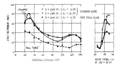
Figure 18: Effect of mass tuning on 5/rev vibratory loads (mastmoment)
