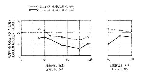
Figure 9: Influence of pendulum weight of a 3/rev blade mounted pendulum absorber on the flapping angle of the absorber
