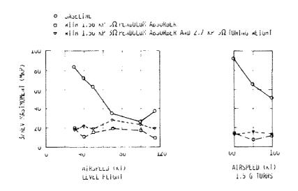
Figure 11: Effect of 3/rev pendulum absorber and 5/rev tuning weight on 3/rev vibratory loads (mastmoment)
