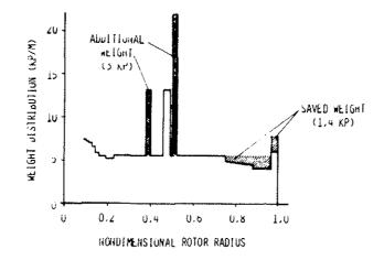
Figure 16: Weight distribution of a vibration treated rotor blade
