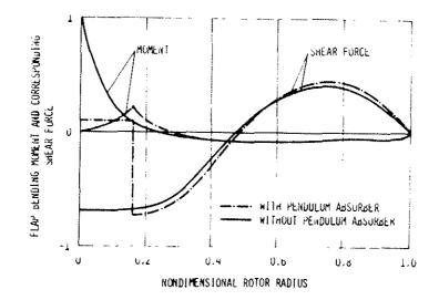
Figure 7: Influence of a 3/rev pendulum absorber on the moment- and shear force distribution of a rotor blade
