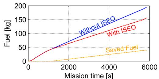
**Fig. 22:** Used fuel of the mission SV 1 with and without ISEO and the saved fuel amount caused by ISEO
