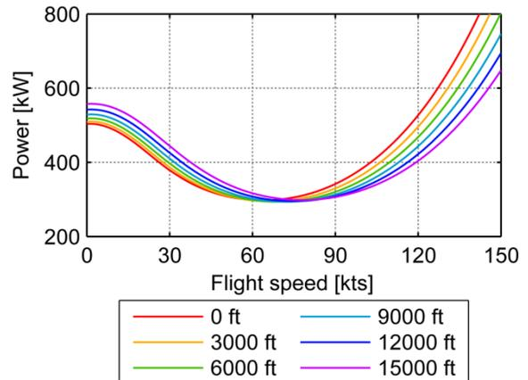
**Fig. 5:** Power required for level flight at different altitudes (flight mass = 2700 kg, ISA conditions,  $H/C_{Ref2}$ )
