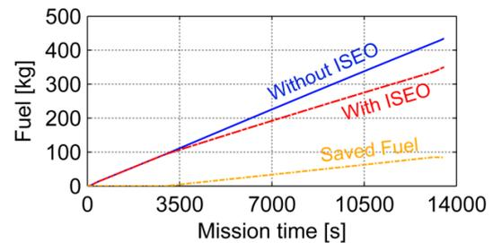
Fig. 25: Used fuel of the mission SV 2 with and without ISEO and the saved fuel amount caused by ISEO
