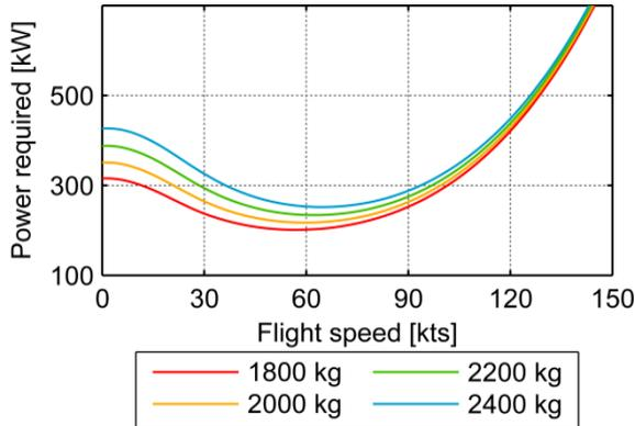
**Fig. 3:** Power required for level flight with different flight masses (MSL, ISA conditions,  $H/C_{Ref1}$ )
