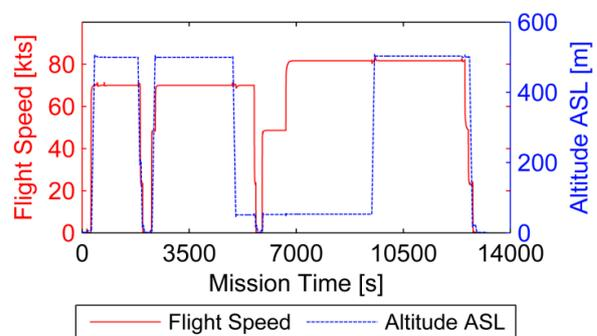
Fig. 26: Flight speed and altitude of the BSN mission
