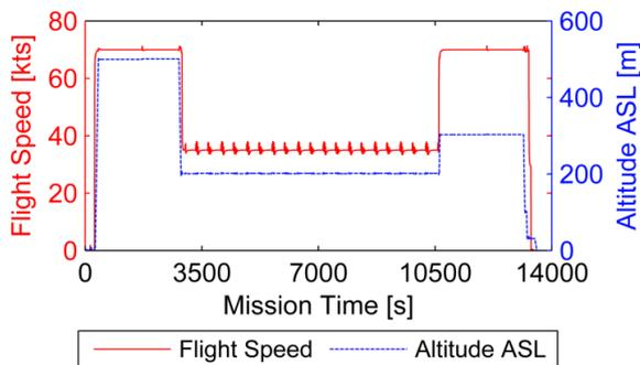
Fig. 23: Flight speed and altitude of the SV 2 mission
