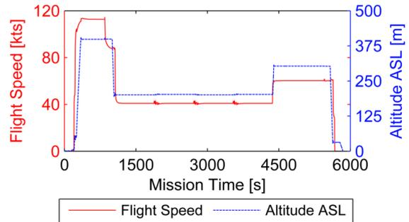
**Fig. 20:** Flight speed and altitude of the SV 1 mission
