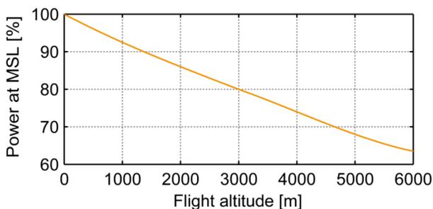
Fig. 2: Percentage MSL power of turboshaft engines at different flight altitudes and ISA conditions
