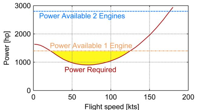
Fig. 1: Typical power required curve (adapted from [5])
