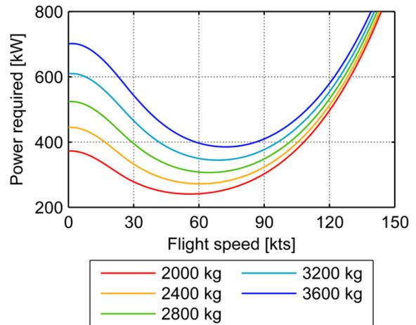
**Fig. 6:** Power required for level flight with different flight masses (MSL, ISA conditions,  $H/C_{Ref2}$ )
