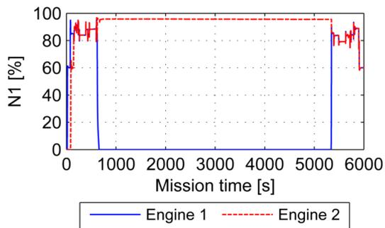
**Fig. 14:** Gas generator spool speed of both engines
