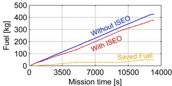
Fig. 28: Used fuel of the BSN mission with and without ISEO and the saved fuel amount caused by ISEO
