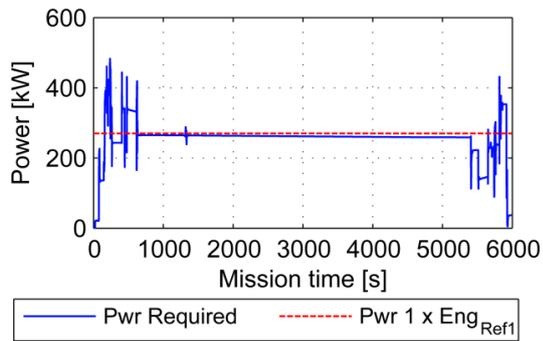
**Fig. 13:** Power required after flight mission parameter modification
