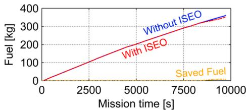
**Fig. 19:** Used fuel of the mission with and without ISEO and the saved fuel amount caused by ISEO
