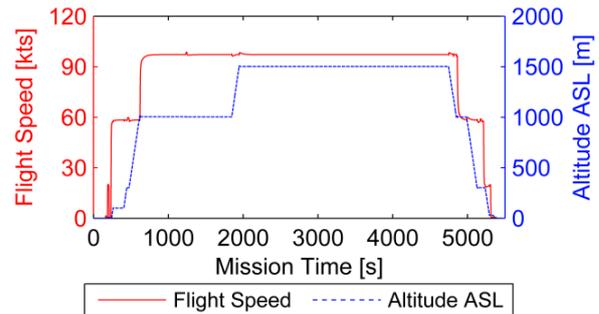
**Fig. 11:** Flight speed and altitude of the OPS mission
