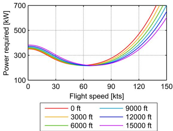
**Fig. 4:** Power required for level flight at different altitudes (flight mass = 2000 kg, ISA conditions,  $H/C_{Ref1}$ )
