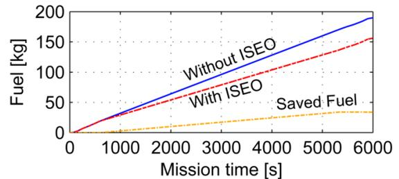
**Fig. 16:** Used fuel of the mission with and without ISEO and the saved fuel amount caused by ISEO
