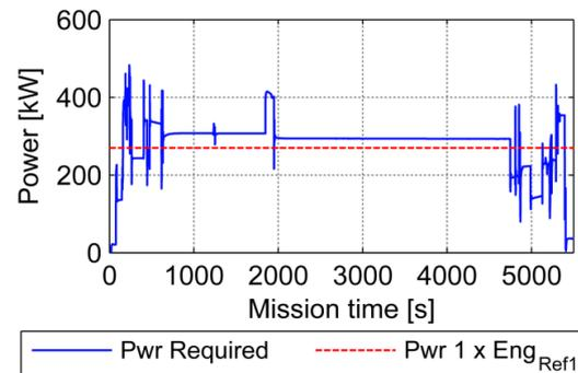
**Fig. 12:** Power required during the OPS mission and power available of one engine
