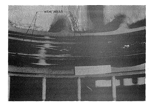
Fig. 6 - Scored Torquemeter Cylinder
