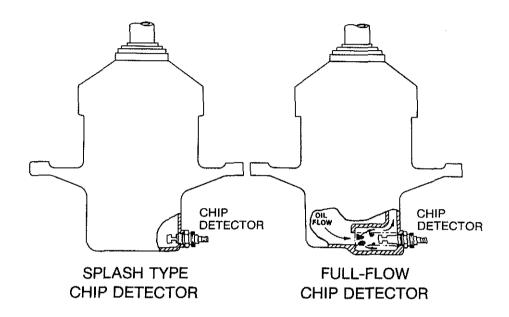
Fig. 1 - Splash-Type Vs. Full-Flow Chip Detection
