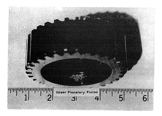
Fig. 3 - Planetary Pinion Bearing Failure
