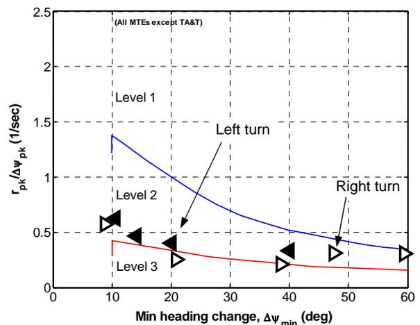
Figure 14: Hover heading quickness from pulse inputs.
