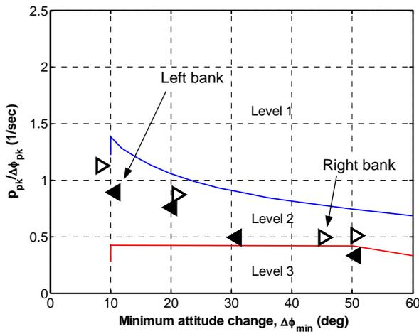
Figure 8: Hover roll attitude quickness from pulse inputs.
