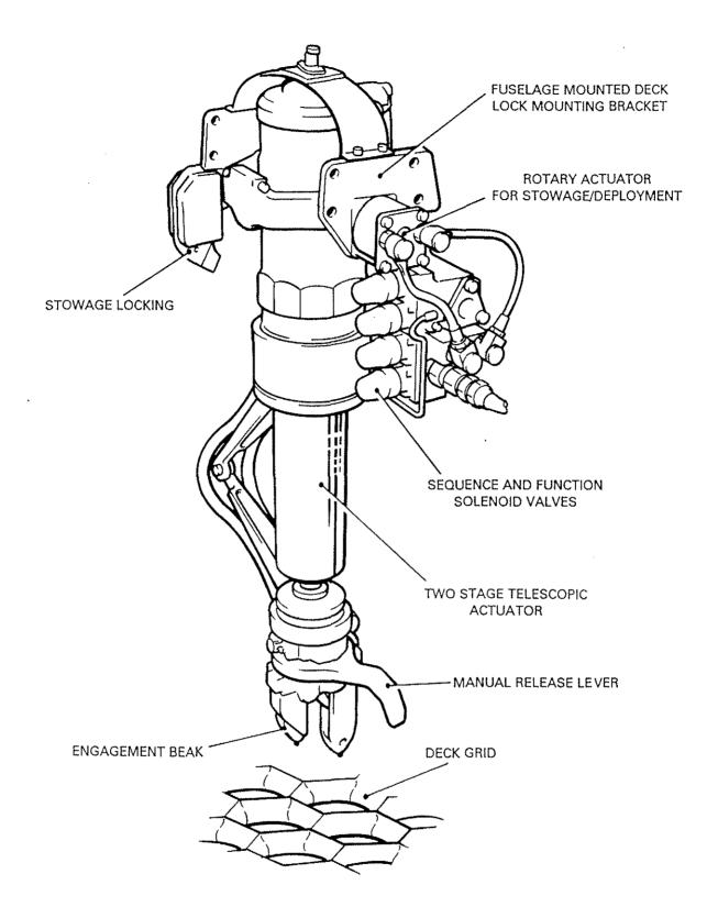
Figure 4 DECK LOCK AND DECK GRID
