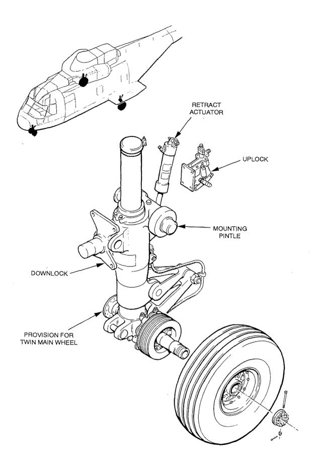
Figure 2 EH101 MAIN LANDING GEAR
