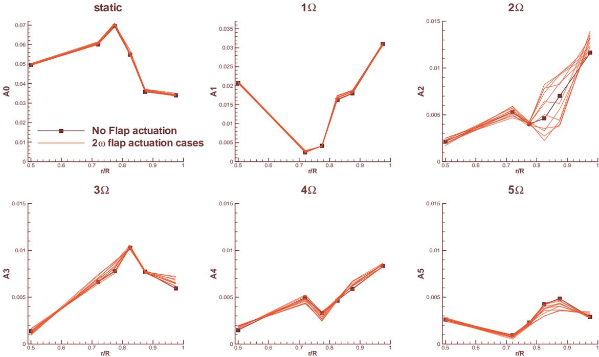
Figure 17 - Harmonic content of the lift coefficient response to several 2-per-rev flaps deflection laws (various phases)
