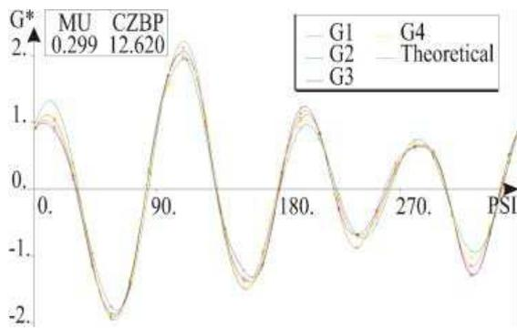
Figure 14 - Comparison theoretical / applied flap deflections
