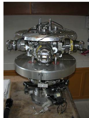
Figure 8 - ORPHEE hub used for ABC tests
