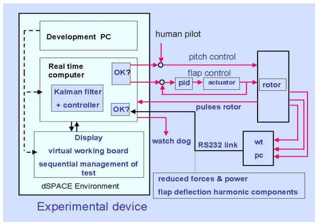
Figure 3 – Flowchart of the active flap control system
