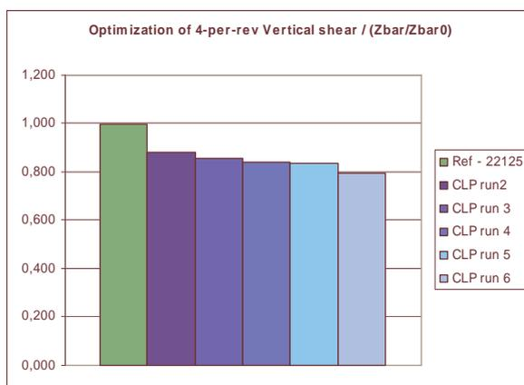
Figure 22 – Vibration reduction thanks to closed-loop optimization
