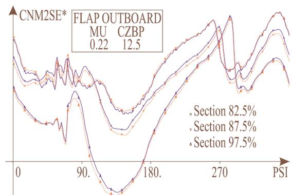
Figure 15 - Repeatability on blade local lift coefficients
