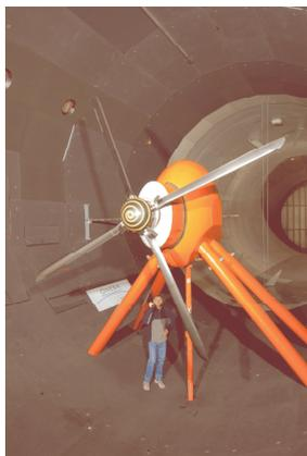
Figure 7 - ABC blades on S1 Modane test rig
