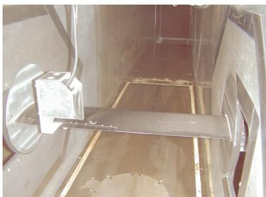
Figure 11 – ABC prototype blade in S3 Modane
