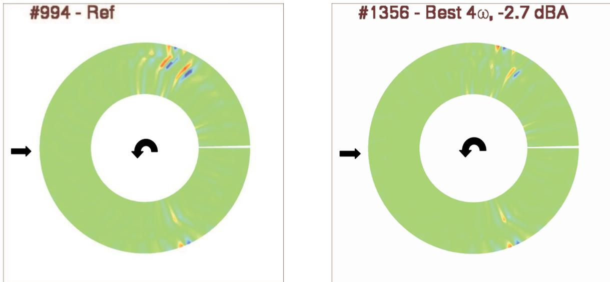
Figure 18 - Comparison of lift coefficient fluctuations measured for a non-actuated case (left) and a case with flap actuation (right)
