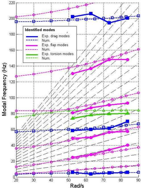
Figure 13 - Comparison theoretical / experimental Campbell diagram
