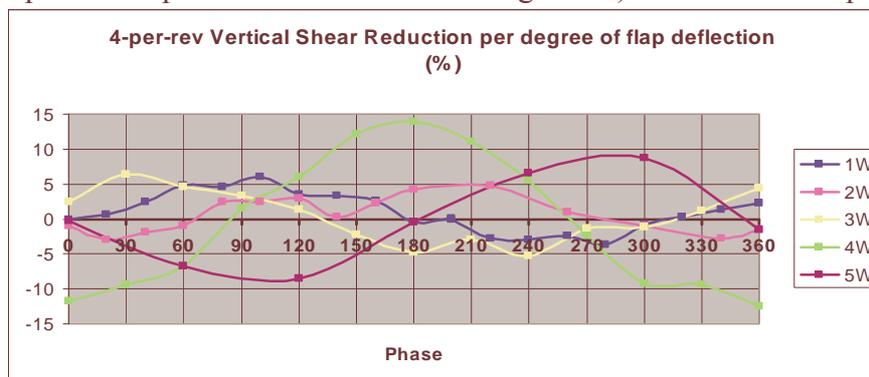
Figure 21 – Sensitivity of 4-per-rev vertical force to harmonic flap deflections
