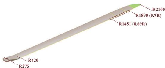
Figure 1 – ABC blade dimensions and flap positions
