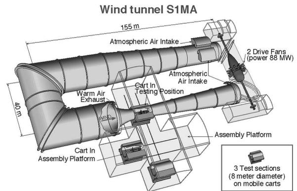
Figure 6 - ONERA S1 Modane wind tunnel
