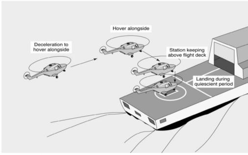
Figure 14: UK RN Standard Deck Landing Approach
