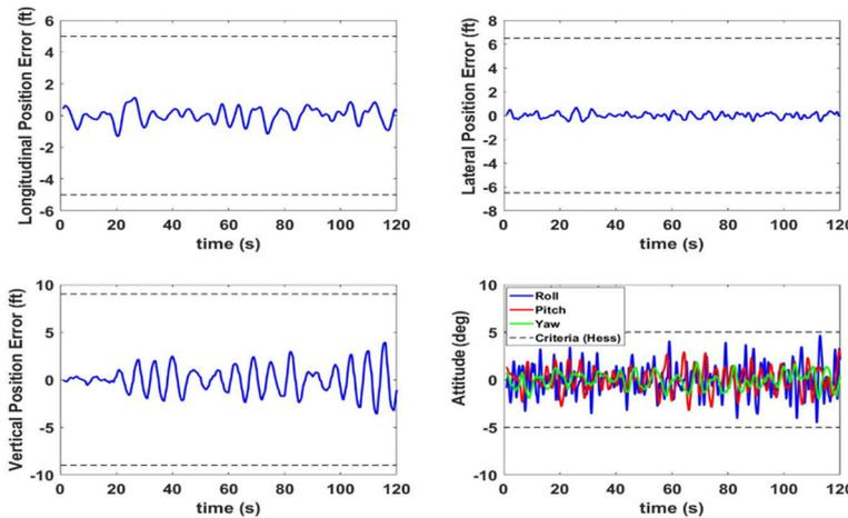
Figure 21: HSDI Pilot Model Task Performance Evaluation through Tracking Errors
