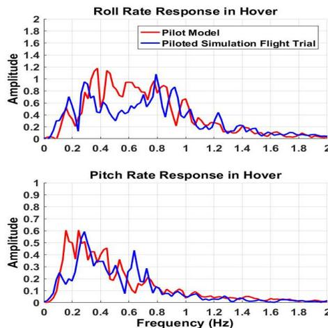
Figure 22: Attitude Rate Response FFT Comparison
