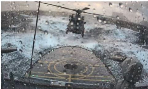
Figure 1: Helicopter Ship Dynamic Interface Environment
