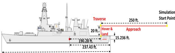
Figure 15: Generic Single-spot Naval Frigate Geometry
