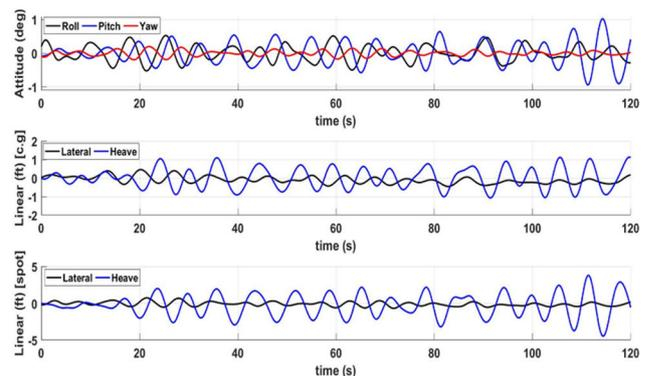
Figure 17: SS4 Ship Motion at c.g. and Landing Spot
