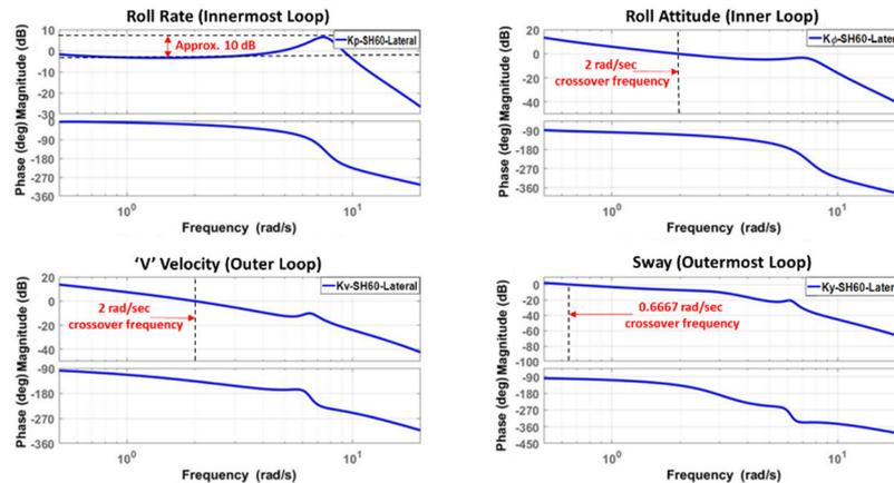
Figure 9: F-D Technique Lateral Channel Pilot Loop Design
