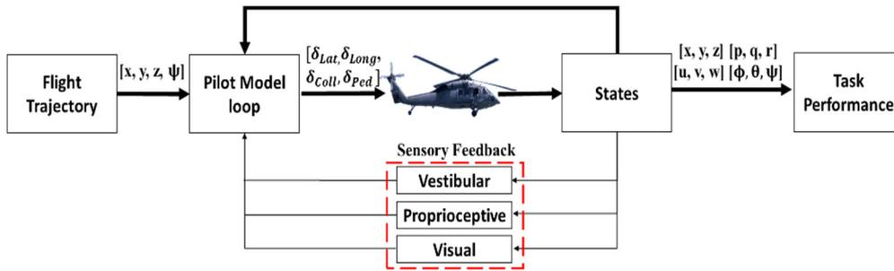
Figure 7: Pilot Model Structure for Motion Sensory Condition
