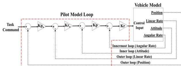
Figure 8: Sequential Pilot Model Loops
