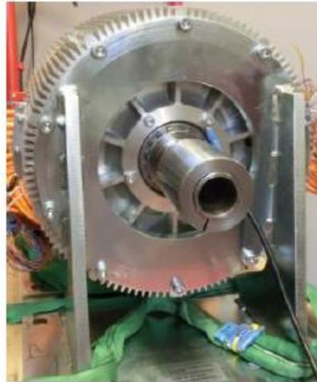
**Figure 2. Axial flux machine with dynamometer mounting arrangement at the University of Bristol**
