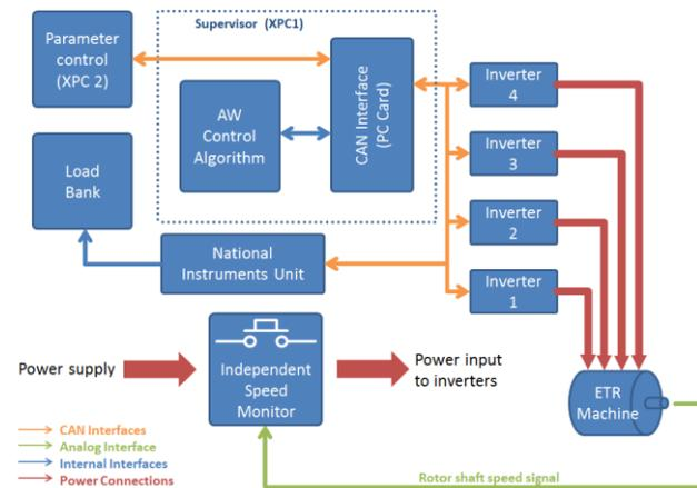
**Figure 21. Control architecture of the grooming rig**
