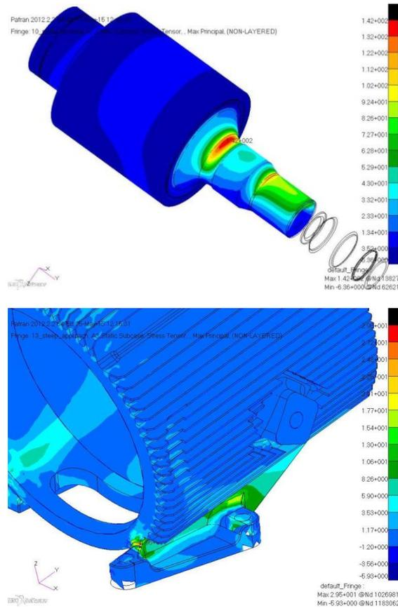
Figure 16. Examples of FE analysis output for the ETR rotor and centre section showing stress contours
