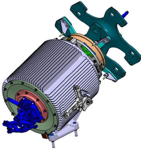
Figure 14. The final ETR machine design. The pitch actuator and tail rotor hub are shown fitted
