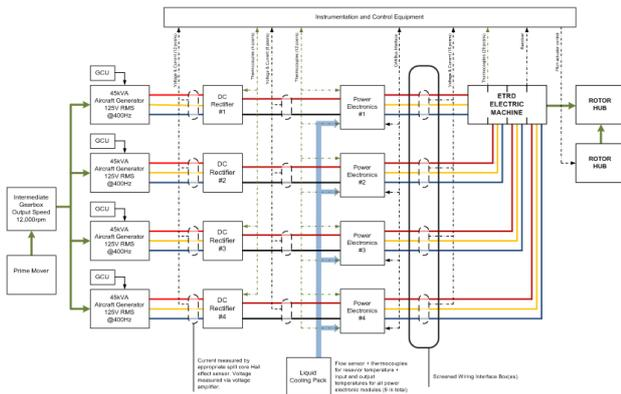
Figure 9. Block diagram of complete ETR electrical system showing the four isolated supplies
