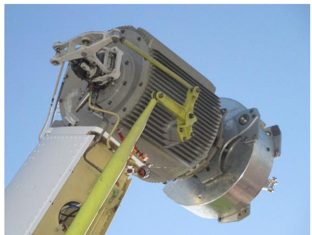
Figure 26. ETR machine installed on the tail fin of the iron bird, along with the pitch actuator and operating mechanism. A hub equivalent mass is fitted to the ETR shaft in preparation for resonance testing
