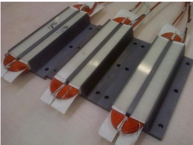
Figure 12. Motorettes before varnish impregnation
