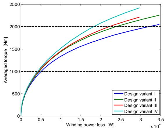
Figure 13. Iterative improvements in efficiency during ETR active component development
