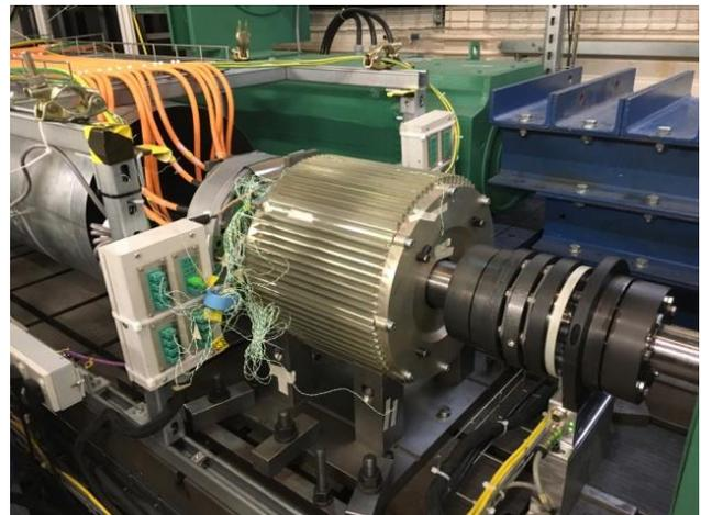
**Figure 3. Radial flux machine undergoing dynamometer testing at the University of Bristol**
