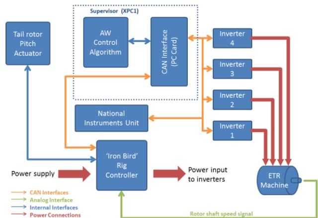
**Figure 22. Control architecture of the Iron Bird rig**
