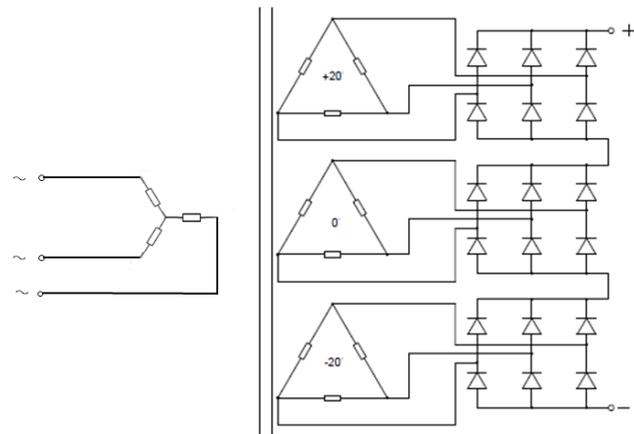
Figure 7. Schematic of phase shifting transformer/ 18-pulse rectifier unit
