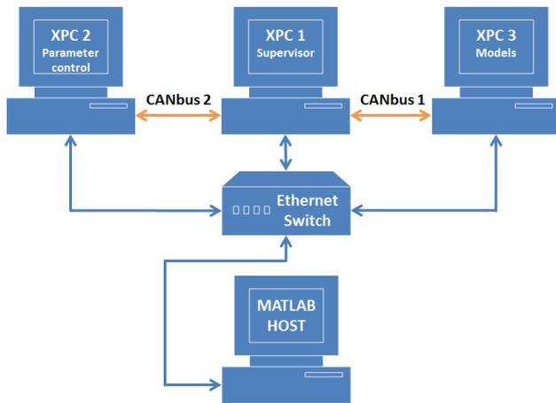
**Figure 20. Control algorithm development environment. The MATLAB host and xPC 3 are not required when controlling the rig**
