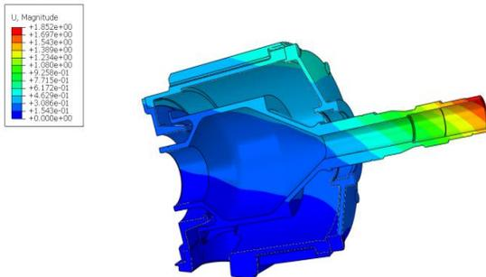
Figure 15. Analysis of stator/rotor air gap
