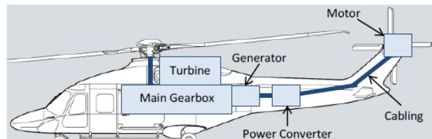
Figure 1. Electric tail rotor basic configuration
