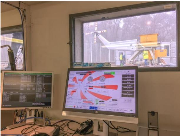
Figure 24. Iron Bird control room. Supervisor display is at left and rig infrastructure display at right. The iron bird rig is visible through the control room window
