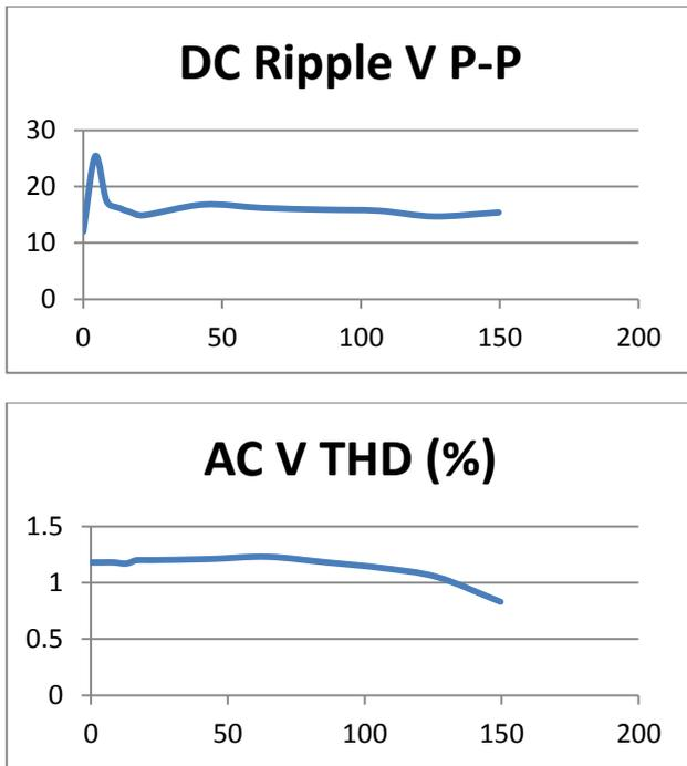
Figure 8. With transformer/18-pulse rectifier in circuit. Top: Ripple on DC output. Bottom: Distortion on input supply, plotted against current
