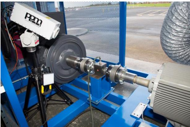
Figure 25. ETR machine (right) coupled to load machine via a torque sensor on the grooming rig
