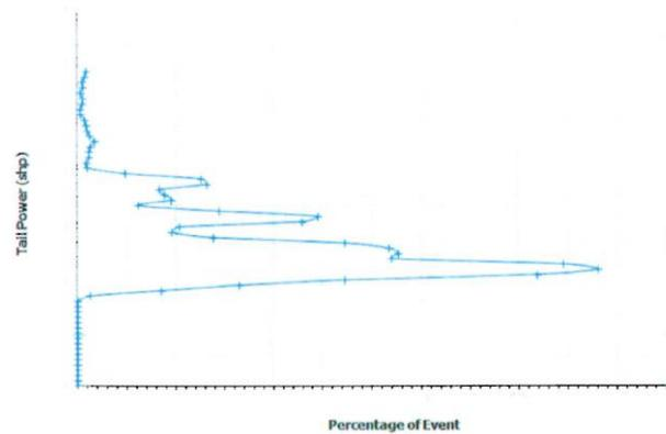
Figure 4. Example of flight test data output showing spread of tail rotor power requirements
