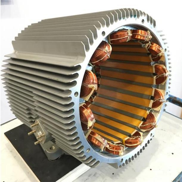
Figure 17. ETR centre section with completed stator
