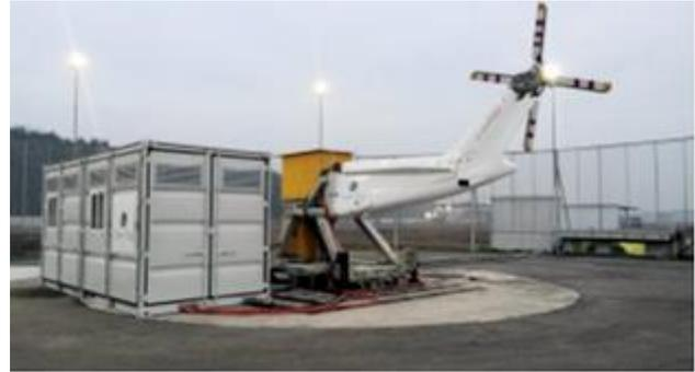
Figure 6. General view of 'Iron Bird' rig
