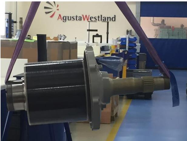
Figure 18. Completed rotor with front end cap fitted to rotor shaft
