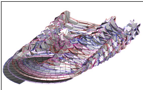
Figure 2 – MESIR wake geometry – descending flight – HART II BL test case
