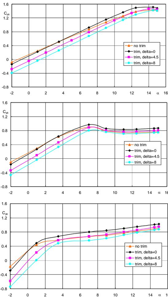
Figure 8.  $C_L(\alpha)$ ;  $M=0.3$  – first line,  $M=0.6$  – second line and  $M=0.8$  – third line
