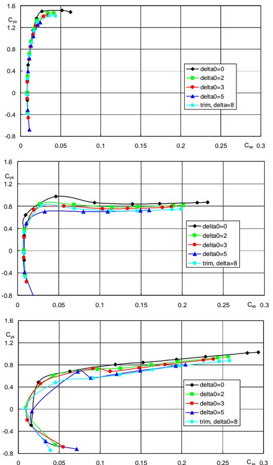
Figure 14.  $C_L(C_D)$ ;  $M=0.3$  – first line,  $M=0.6$  – second line and  $M=0.8$  – third line
