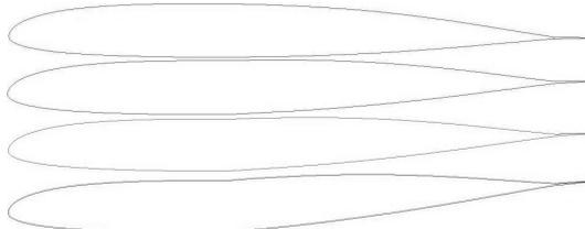
Figure 3. Geometry of KS profile with tail section deflected on  $\delta=0, 2^\circ, 3^\circ, 5^\circ$
