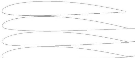
Figure 4. Geometry of SB profile without trim tab and with trim tab deflected on  $\delta=0, 6^\circ, 8^\circ$
