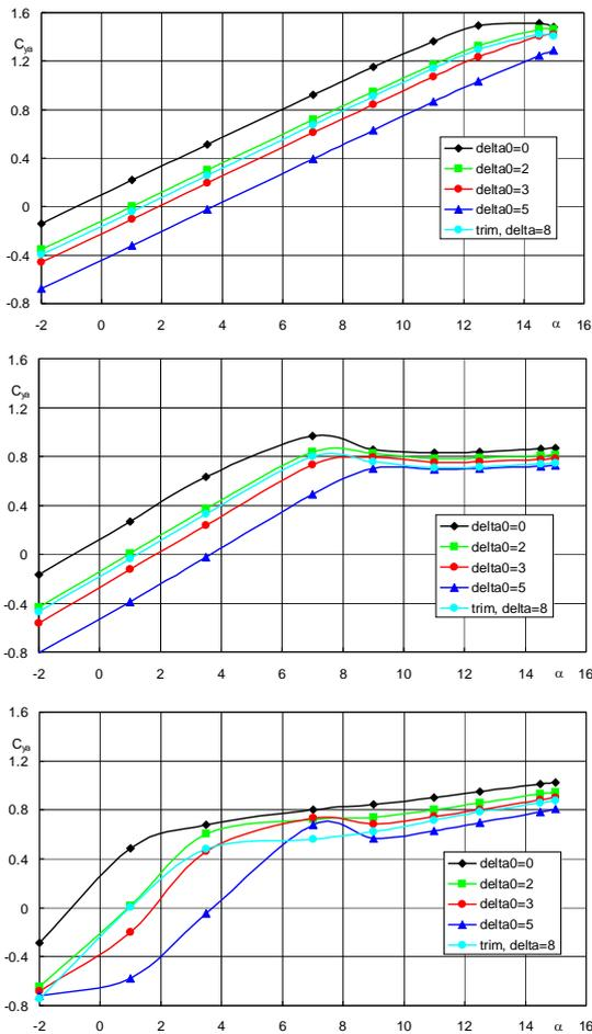
Figure 13.  $C_L(\alpha)$ ;  $M=0.3$  – first line,  $M=0.6$  – second line and  $M=0.8$  – third line
