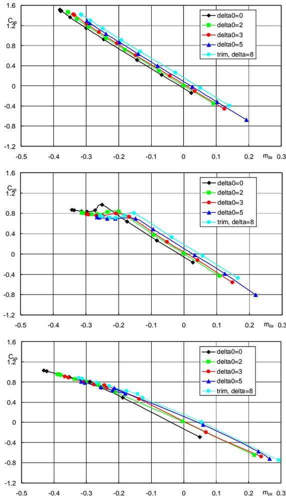
Figure 15.  $C_L(m_z)$ ;  $M=0.3$  – first line,  $M=0.6$  – second line and  $M=0.8$  – third line
