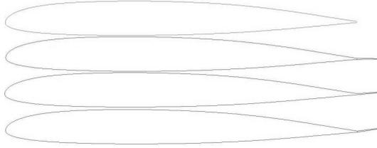
Figure 2. Geometry of KS profile without trim tab and with trim tab deflected on  $\delta=0, 4.5^\circ, 8^\circ$
