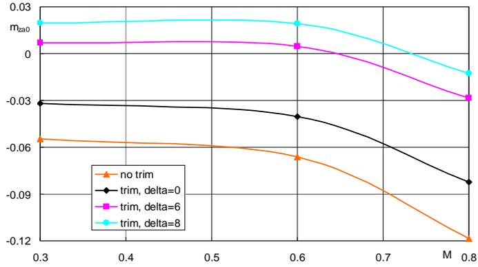
Figure 12.  $m_{z0}$  for different Mach number, SB profile
