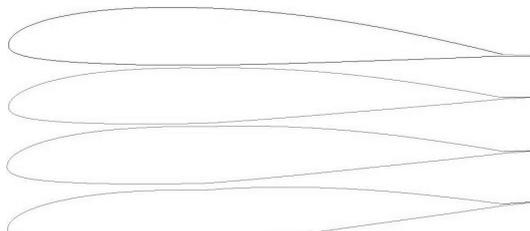
Figure 5. Geometry of SB profile with tail section deflected on  $\delta=0, 2^\circ, 3^\circ, 5^\circ$
