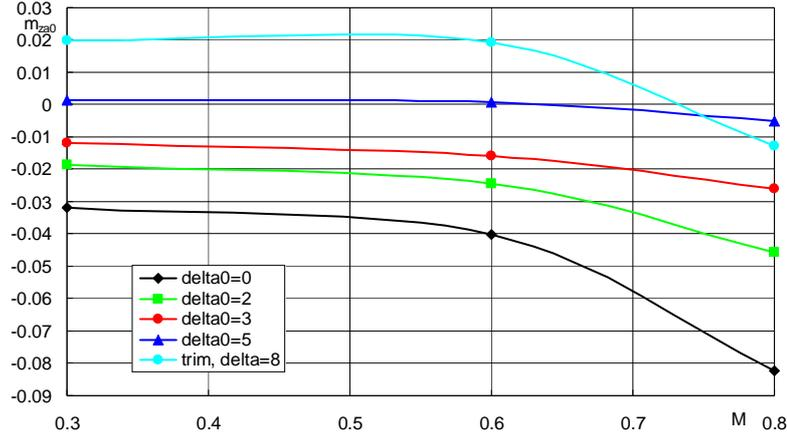
Figure 17.  $m_{z0}$  for different Mach number, SB profile
