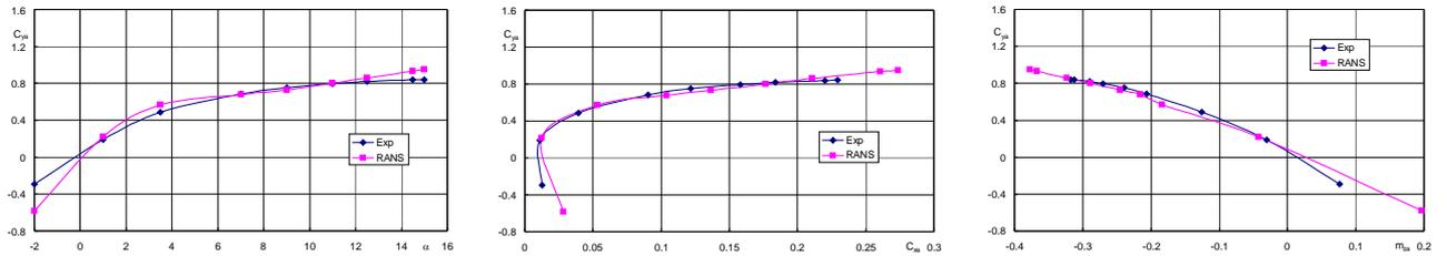
Figure 7. Comparison of calculated (magenta) and experimental (blue) data:  $C_L(\alpha)$ ,  $C_L(C_D)$  and  $C_L(m_z)$
