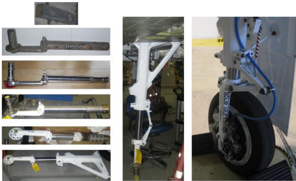
Figure 20. Production of demonstration aerospace components from Ferrium S53 —T-38 main landing gear piston.
