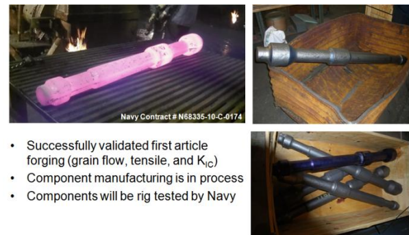
Figure 14. Ferrium M54 T-45 Goshawk hookshank forging.
