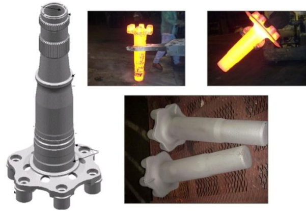
Figure 7. Ferrium C61 prototype CH-47 Chinook helicopter forward rotorshaft production (Army Phase II SBIR contract #W911W6-10-C-0057). A projected potential weight savings of 15–25% is expected over the incumbent shaft material.
