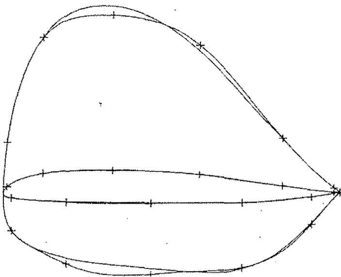
Fig.3. Initial TsAGI helicopter airfoil compared with designed airfoil.
