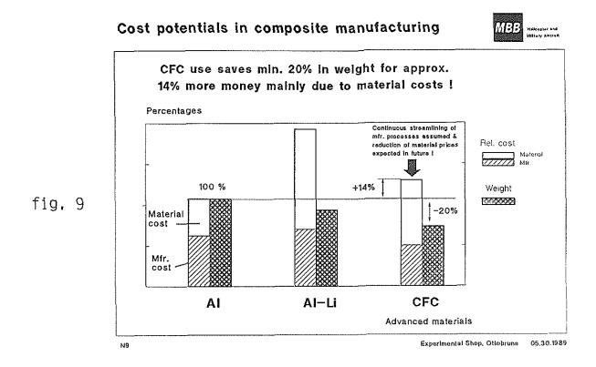
After this introduction, I would like to compare the productioncost calculation of identical structures both in metal (here: Aluminium alloy) and carbon fibre reinforced plastic. According to this calculation, we have to assume that a lightweight structure made with carbon fibres is still more expensive today, mainly due to the high material prices.
