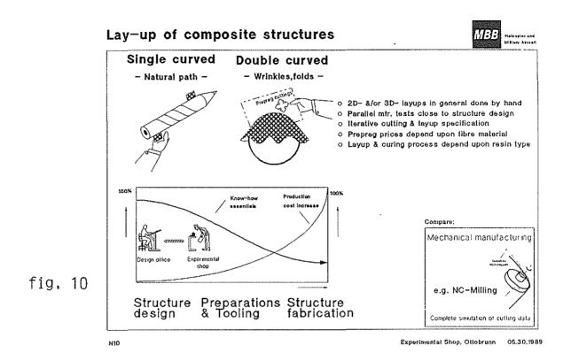
The core operation of composites manufacturing is very similar to an assembly process, where different parts have to be positioned and fixed in a given orientation. As you probably remember, this lay-up of fabric-cuttings cannot be completely simulated on drawing boards or design screens if the loft or surface of the composite parts is curved. Furthermore, the draping of a flat cutting on a curved surface will follow a natural path and will eventually fall in folds.
