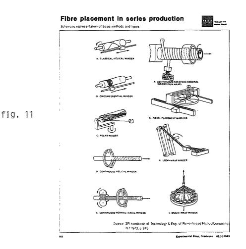
This figure shows well known methods and types of mechanical fibre placement in composites manufacturing. What all these kinematic solutions have in common is that we have a continous lay-up process with endless rovings or tapes and that they can be profitably used to manufacture flat or convex parts with closed surfaces.
