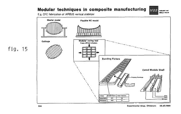
I assume that we all know the modular or unit construction principle very well from many designs of structures and equipment both in aerospace products as well as in tooling. Regarding the variety of composite structures and toolings, however, I feel that this idea should be taken up again by the production engineers.
