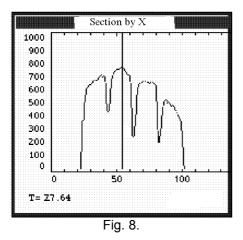
The MR torsion heating under cyclic tests was studied with the aid of a thermal imaging radiometer. The temperature values in the torsion transverse direction are presented in Fig. 8.
