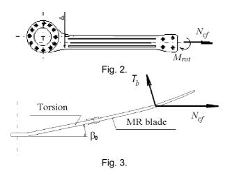
A special feature of the hub structure is the fact that the torsion housing which transfers a torque and controlling actions from the blade to the wobble plate bears no tensile and bending loads owing to the kinematic scheme of torsion attachment.
