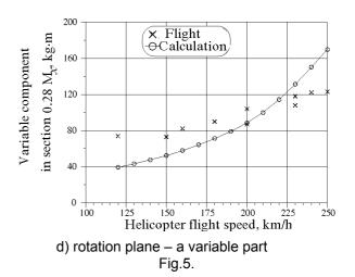
Figure 5 presents the standard calculation and experimental data on bending moments in the flapping plane (a) and rotation plane (b) depending on flight speed.
