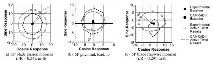
Figure 23. Comparison of CAMRAD II and experimental 5P rotating-system response to 5P, 1000 V IBC actuation.  $\mu$  = 0.140,  $C_L$  = 0.0066,  $\alpha_s$  = -1.0°.
