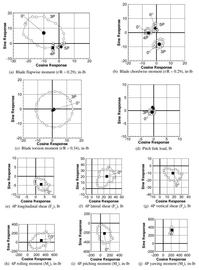
Figure 8. Rotating- and fixed-system response maps for  $\mu$  = 0.140,  $C_L$  = 0.0066,  $\alpha_s$  = -1.0°, and 3P, 1000 V IBC actuation.
