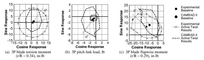
Figure 21. Comparison of CAMRAD II and experimental 3P rotating-system response to 3P, 1000 V IBC actuation.  $\mu = 0.140$ ,  $C_L = 0.0066$ ,  $\alpha_s = -1.0^\circ$ .
