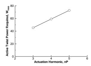
Figure 20. Rotor actuation power required.
