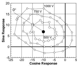
Figure 7. Sample response map or "circle plot." Blade flapwise bending moment (0.29R) for 3P IBC control.  $\mu$  = 0.140,  $C_L$  = 0.0066,  $\alpha_{\rm s}$  = -1.0°, and 1000 V actuation.
