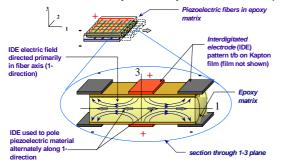
Figure 4. Active Fiber Composite (AFC) piezoelectric actuator concept.
