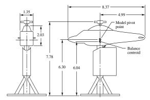
Figure 2. Schematic of the Aeroelastic Rotor Experimental System (ARES) helicopter testbed. All dimensions are in feet.
