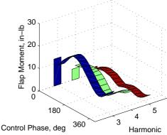
Figure 5. Sample ribbon plot. Blade flapwise bending moment (0.29R) for 3P IBC control.  $\mu$  = 0.140,  $C_L$  = 0.0066,  $\alpha_s$  = -1.0°, and 1000 V actuation amplitude.
