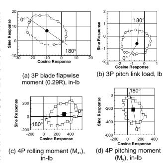
Figure 11. Rotating- to fixed-system loads comparison for  $\mu$  = 0.140,  $C_L$  = 0.0066,  $\alpha_{\rm s}$  = -1.0°, and 3P, 1000 V IBC actuation.
