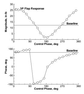
Figure 6. Sample response plot. Blade flapwise bending moment (0.29R) for 3P IBC control.  $\mu$  = 0.140,  $C_L$  = 0.0066,  $\alpha_s$  = -1.0°, and 1000 V actuation.
