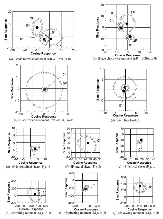
Figure 10. Rotating- and fixed-system response maps for  $\mu$  = 0.140,  $C_L$  = 0.0066,  $\alpha_s$  = -1.0°, and 5P, 1000 V IBC actuation.
