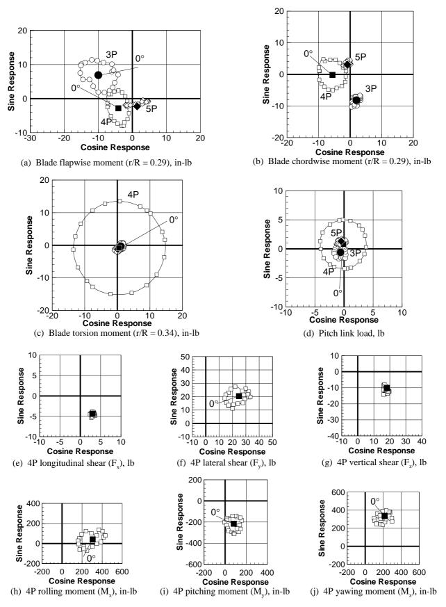
Figure 9. Rotating- and fixed-system response maps for  $\mu$  = 0.140,  $C_L$  = 0.0066,  $\alpha_s$  = -1.0°, and 4P, 1000 V IBC actuation.
