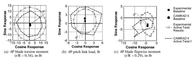
Figure 22. Comparison of CAMRAD II and experimental 4P rotating-system response to 4P, 1000 V IBC actuation.  $\mu$  = 0.140,  $C_L$  = 0.0066,  $\alpha_s$  = -1.0°.
