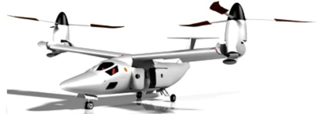
Figure 12 University of Maryland's "Excalibur", Variable Diameter Tiltrotor aircraft.
