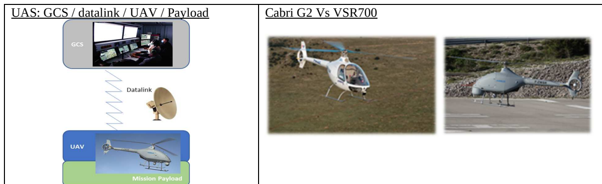
Figure 1 : UAS definition. Cabri G2 compared to VSR700
