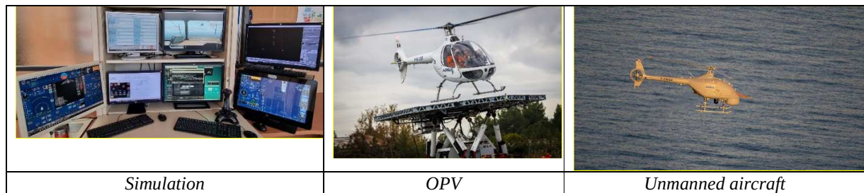
Figure 10: Test strategy for flight controls
