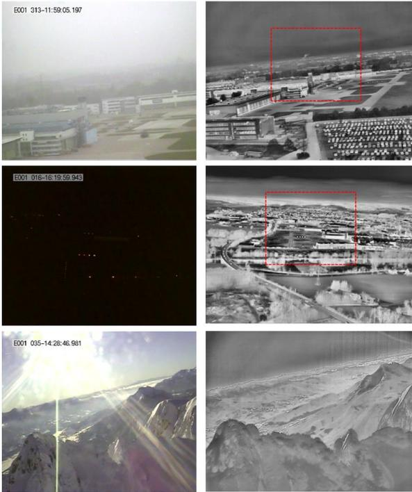
Fig. 11: HeliEVS (right) and corresponding daylight camera recording (left) under foggy, night and bright sunlight conditions
