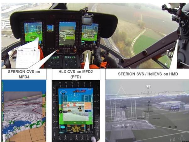
Fig. 2: DVE Cockpit displays in H145
