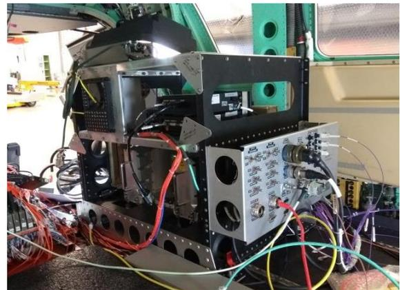
Fig. 10: DVE System rack in the cabin
