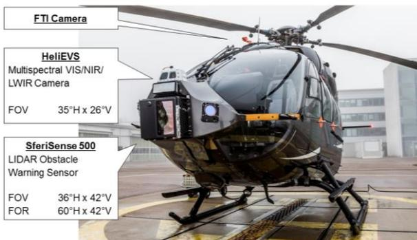
Fig. 9: DVE Sensor assembly on H145
