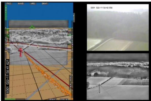
Fig. 12: SferiAssist MFD output (left) with corresponding FTI camera (upper right) and HeliEVS image (lower right)
