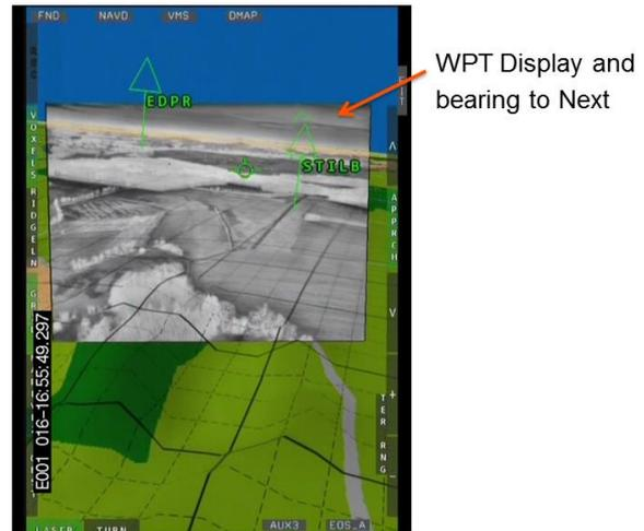
Fig. 5: Navigation Support with SferiAssist CVS
