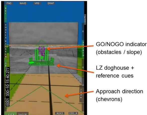
Fig. 6: Take-off and Landing Support with SferiAssist CVS
