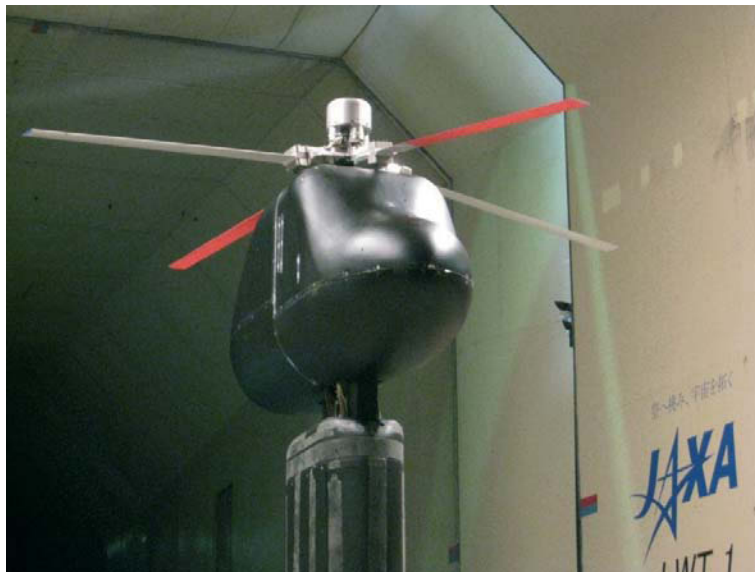
Figure 1: Photograph of JMRTS in JAXA 6.5mx5.5m Low-Speed Wind Tunnel
