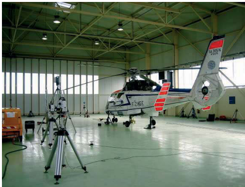
Figure 17: Positioning of the sensors in the helicopter frame
