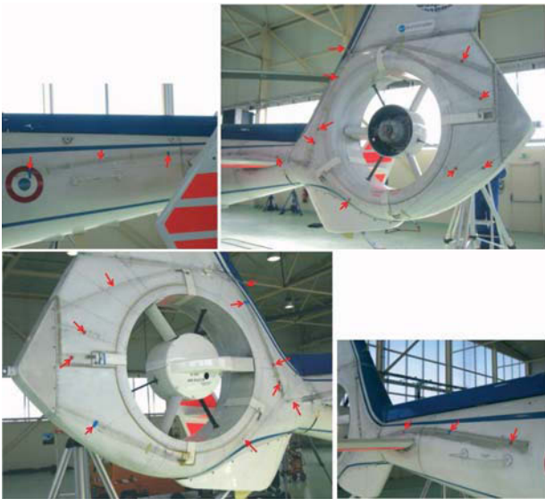
Figure 6: Position of the pressure measurements
