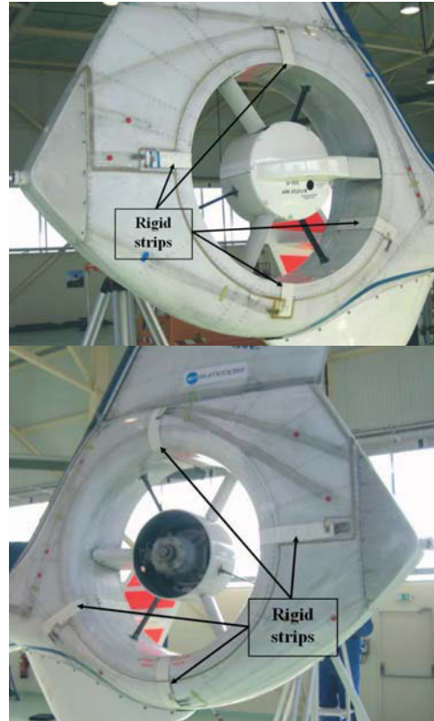
Figure 7: Position of the rigid strips around the Fenestron
