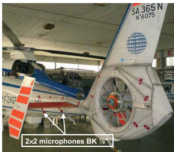
Figure 2: Implementation of the microphones
