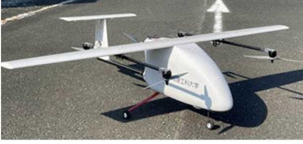
Figure 1: Scaled-down model of a lift + cruise type eVTOL aircraft under test in SIST.
